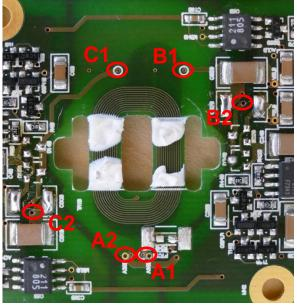
Figure 3: Measurement points on the DUT
