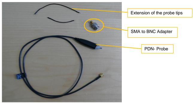
Figure 4:One-Port PDN Probe from Picotest
