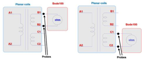
Figure 9Inner Coil Measurement B and C
