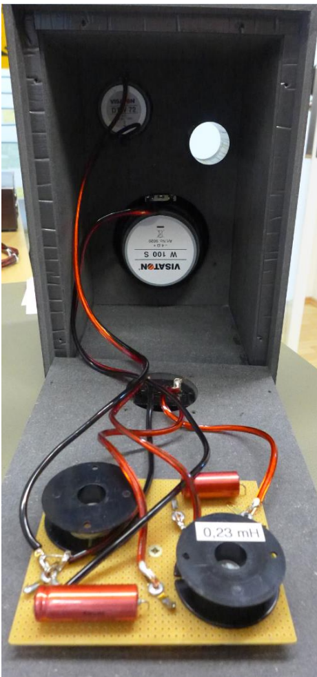
Figure 1: Satellite speaker including tweeter, mid-range driver and audio crossover
