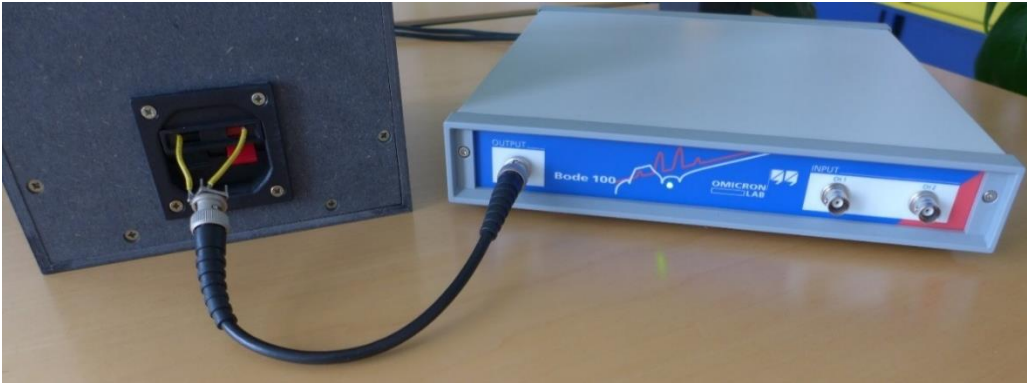
Figure 4: Impedance measurement of the loudspeakers
