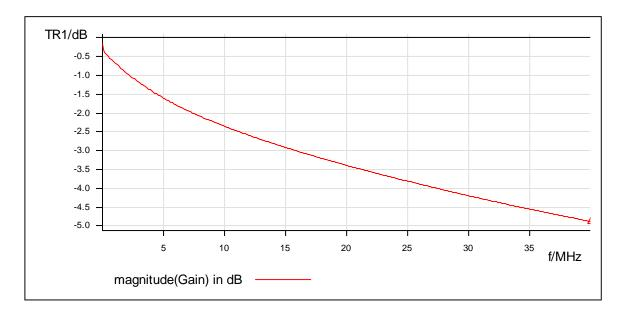
Connect one cable end to the Bode 100 output and the other cable end to the CH2 of the Bode 100. A sweep shows the following result:
