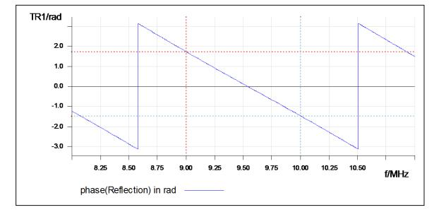
• Shift both cursors to advantageous frequencies and read the values  $\Delta \Phi = -3.20 \text{ rad}$  $\Delta f = 1.0 \text{ MHz}$
