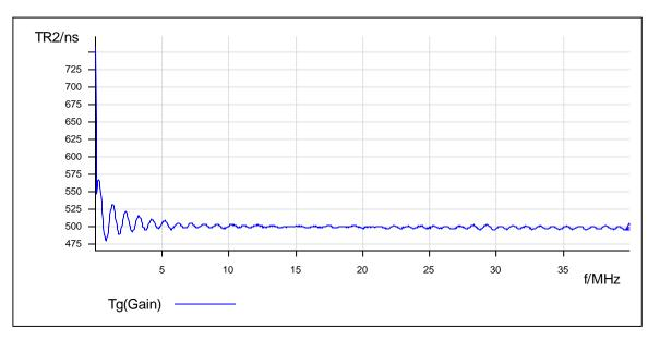
When you have a closer look at the measured curve you immediately detect a ripple. This ripple is caused by the fact that the wave impedance of the cable is not exactly 50 Ohms. The ripple amplitude increases the lower the frequency gets since the series impedance of the cable becomes more dominant at lower frequencies.
