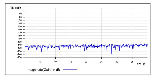
As you can see in the chart above the isolation between the double shielded cables is much better (attenuation > 100dB)
