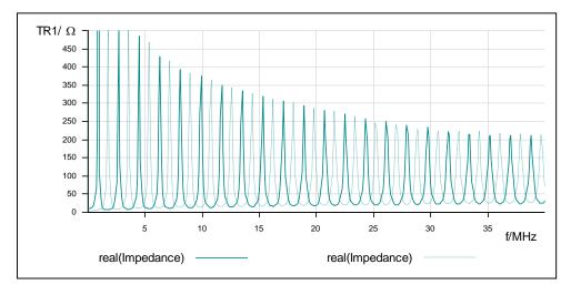
• Diagram for the measured impedance of a 75Ω cable (50 meters):
