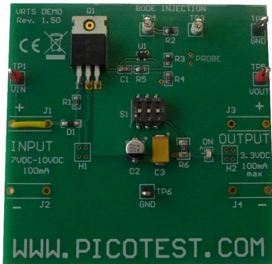
Figure 1: Voltage Regulator Test Standard board (VRTS 1.5)
