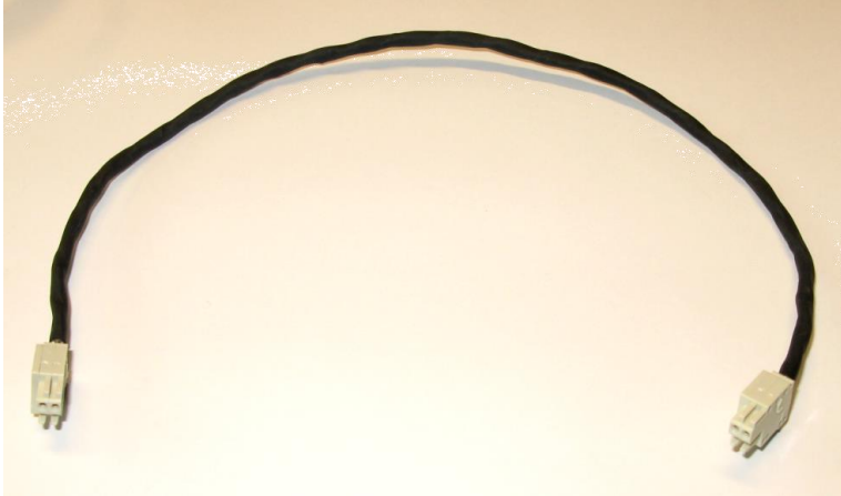
Figure 5: Calibration cable for THRU calibration
