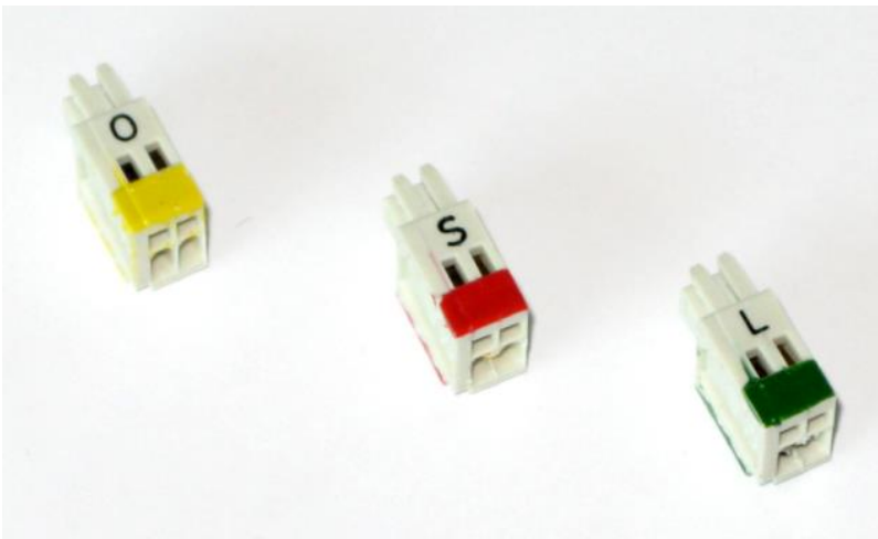
Figure 4: OPEN, SHORT, LOAD calibration connectors
