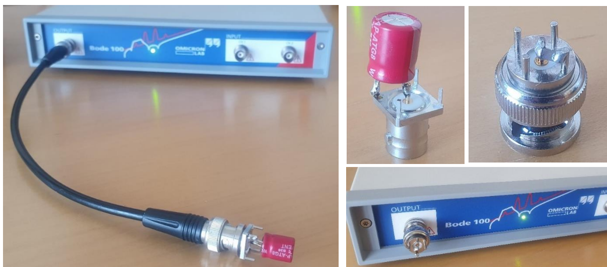
Figure 13: One-Port – solder DUT to BNC
