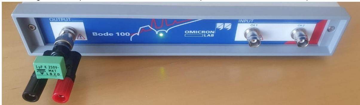
Figure 14: One-Port – connect to BNC adapter
