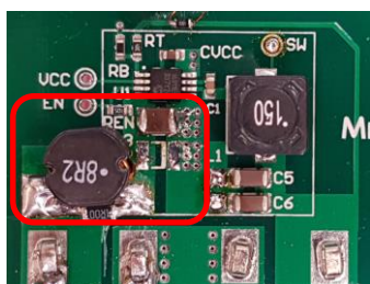
Figure 7: DC/DC converter with mounted input filter
