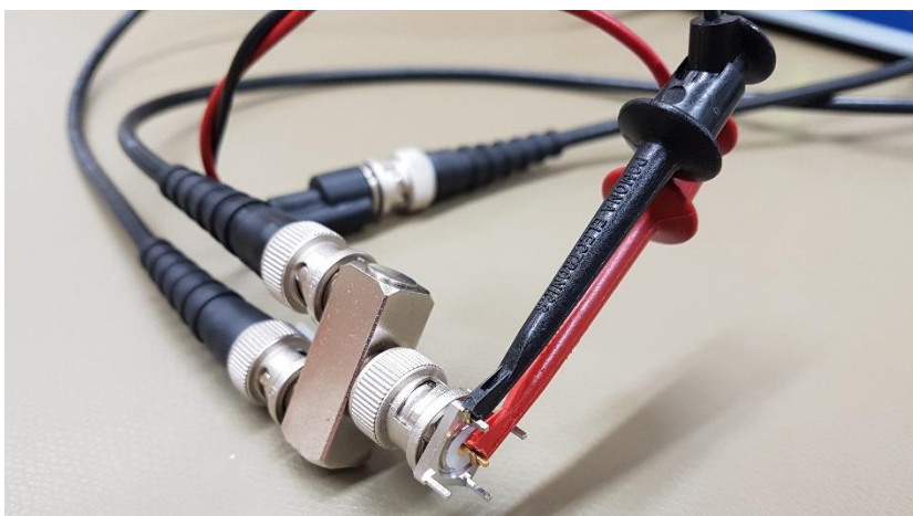
Figure 8: close-up of the connection for the THRU calibration
