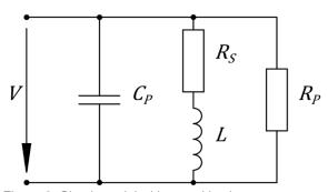
Figure 2: Circuit model with parasitic elements
