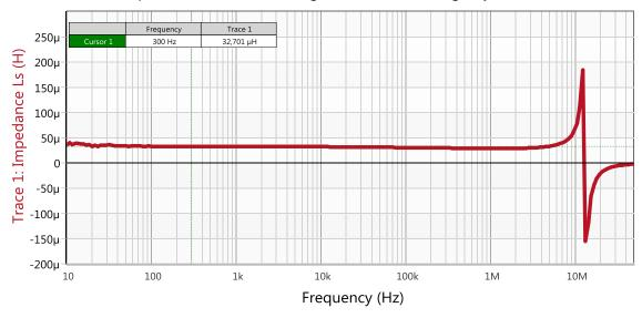
Figure 13: Measurement result - inductance
