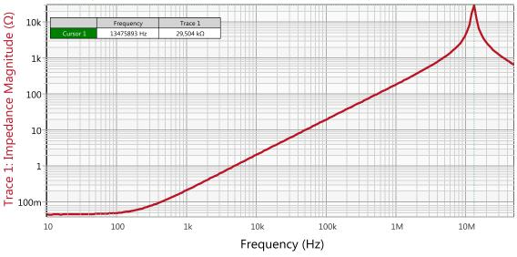
Figure 14: Frequency sweep over the whole frequency range
