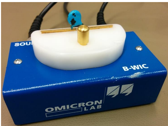
Figure 24: Y capacitor measurement with B-WIC Impedance Adapter
