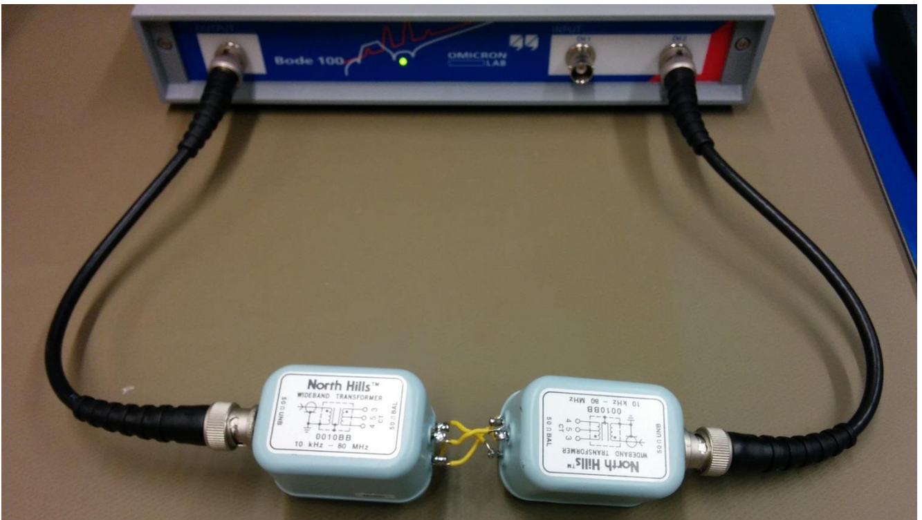
Figure 13: Differential mode Thru-calibration
