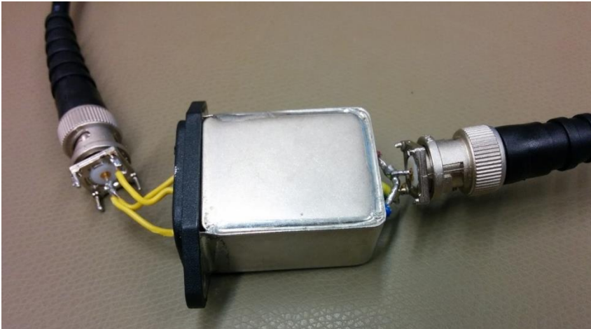
Figure 9: Common mode connection with BNC connectors
