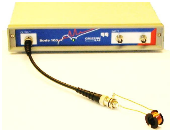
Figure 3: Setup for the self-inductance measurement
