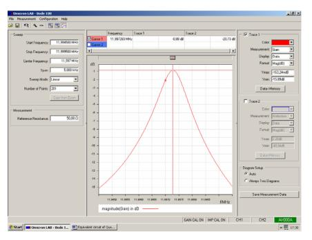
Using the cursor 1 and cursor 2 we get fs = 11.997339MHz and  $B_{3dB}$  = 978Hz and  $Q_L$  = 12267 Finally we have to measure the Series Resistance  $R_S$  to calculate Q of the crystal. One possibility is to use the measured attenuation at the Series resonant frequency, the other way is to measure the impedance of the crystal at the Series resonant frequency.
