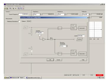
Open the Calibration window and perform the impedance calibration by measuring "Open", "Short" and "Load" as described in the Bode 100 user manual.
