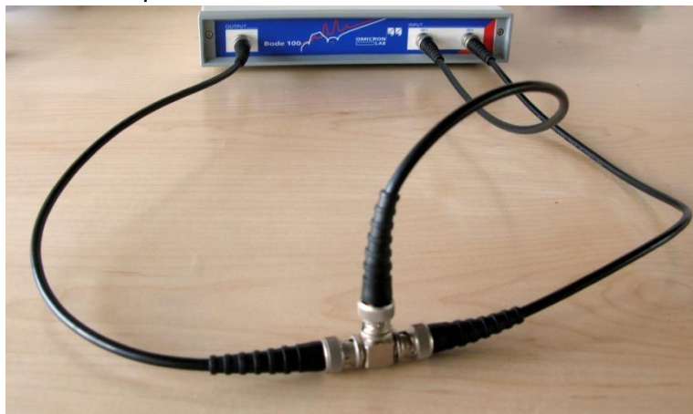
Figure 14: gain/phase accuracy - connection setup
