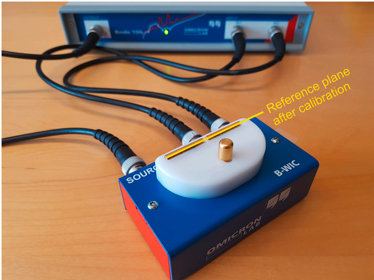
Figure 10-6: Calibrating the B-WIC impedance test fixture by performing Open, Short and Load Calibration
