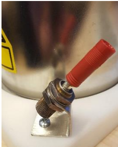
Figure 1 Connection of 6mm to 4mm reducer plug to CP TC12 oil test cell
