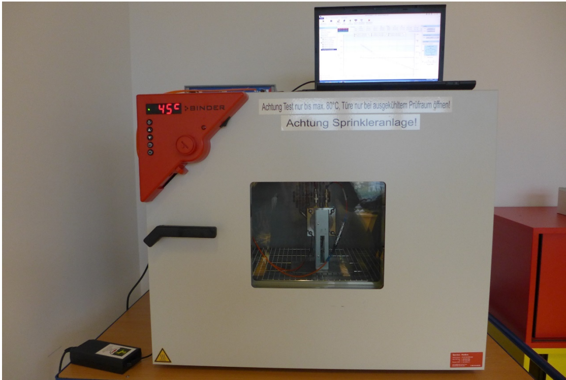
Figure 1: Dielectric material analysis using the Liquid Test Fixture 16452A from Keysight - Setup
