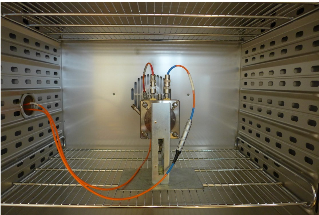
Figure 2: Dielectric material analysis using the Liquid Test Fixture 16452A from Keysight - Connection
