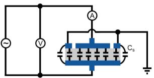
Figure 5: Measurement circuit, guarded electrode (Cs is stray capacitance)
