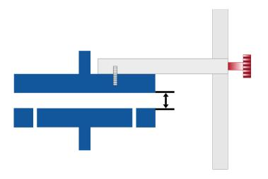
Figure 8: Adjusting the air gap height by using a locking screw
