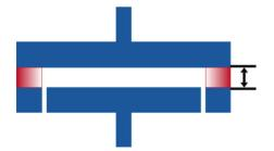
Figure 7: Adjusting the air gap height by using a spacer
