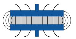
Figure 3: Lines of electric force, unguarded electrode<sup>2</sup>
