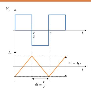
$$L[H] = \frac{\Phi[Vsec]}{I_{PP}[A]} = \frac{V_{rms}}{I_{PP}} \frac{T}{2} = \frac{V_{rms}}{I_{PP}} \frac{1}{2f} = \frac{U dt}{di}$$
