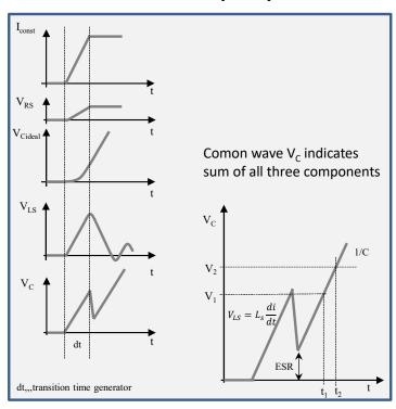
DC-Impedance is more directly related to device behavior in many pulse power applications
