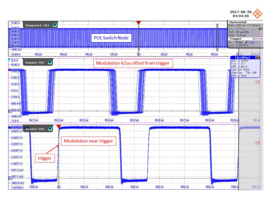
Many switching power supplies use less than stellar oscillator circuits, resulting in switching frequency jitter
