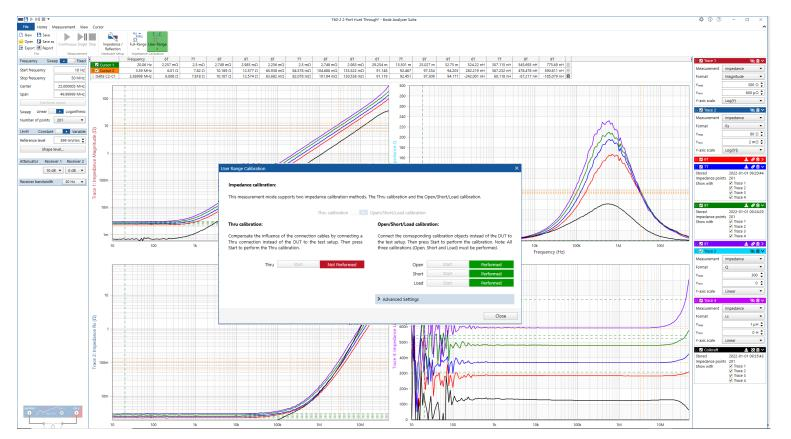
Frequency Domain (VNA) allows very simple and accurate calibration to correct for cable probe errors
