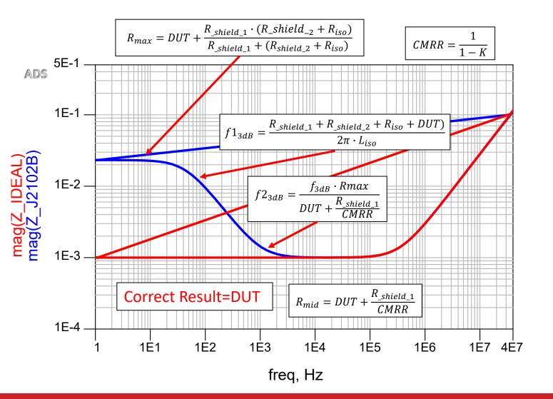
The transformer isolator is complex, but depends on excellent coupling for high CMRR, high isolation inductance and low DC resistance
