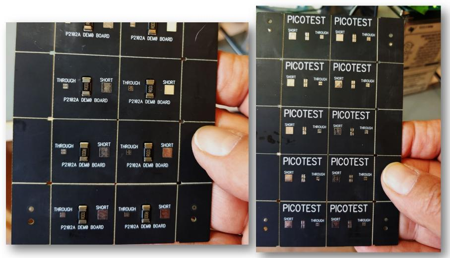
A 1 milliohm resistor is mounted on the topside of this demo board
