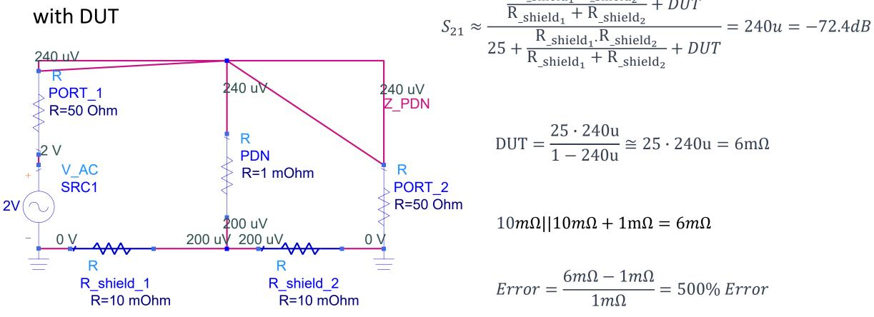
$R_{\underline{shield_1}}$ . $R_{\underline{shield_2}}$  + DUT
