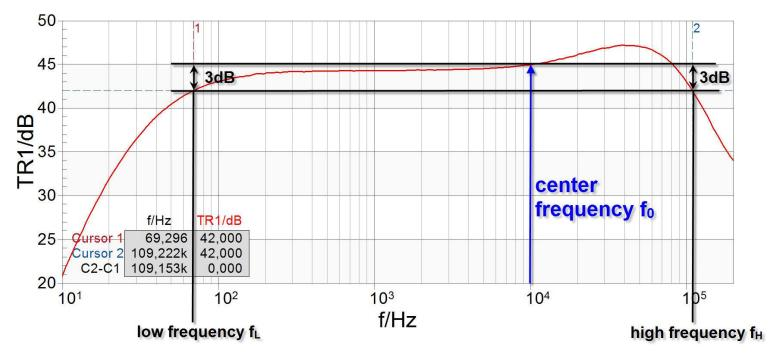
Audible frequencies range from 20 Hz to 20 kHz  $\rightarrow$  center frequency f<sub>0</sub> @ 10 kHz chosen
