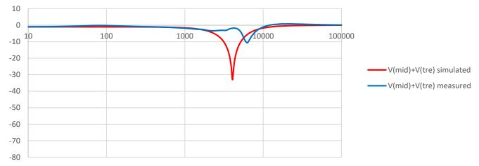
Comparison diagrams created in Excel<sup>®</sup> by copying the trace data from the BAS and exporting the LTspice simulation curves.
