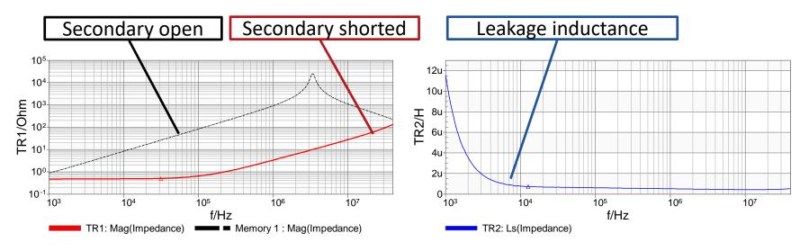
$\rightarrow$  Leakage inductance is not constant over frequency
