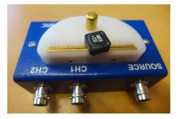
$$\begin{split} H &= 33 \mu H \ (\pm 20\%) \ @ \ 1 \ kHz \\ R_{DC} &= 0,049 \ \Omega \ (typ.) \\ R_{DC} &= 0,057 \ \Omega \ (max.) \\ f_{res} &= 11 \ MHz \end{split}$$
