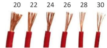
Secondary rms current sizes the wire gauge
