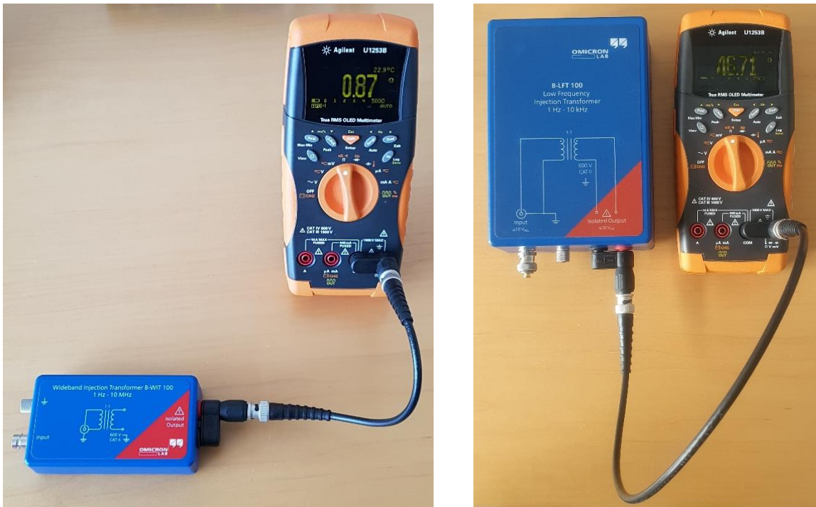
Figure 2: Measurement setup - DC resistance of output
