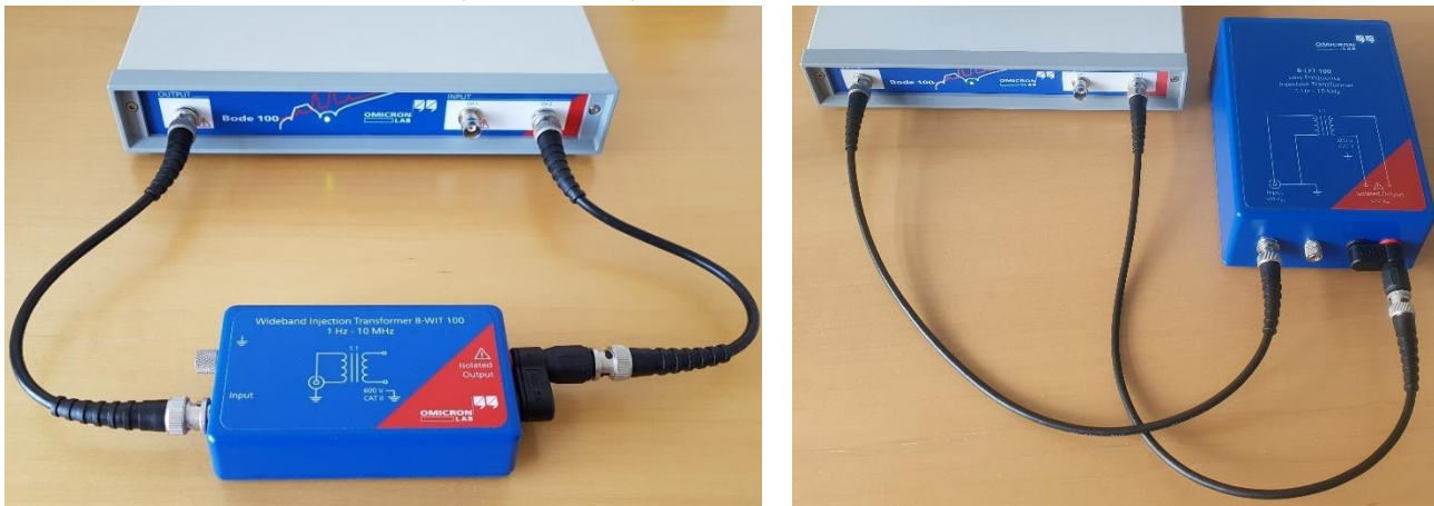
Figure 4: Measurement setup - check of frequency range
