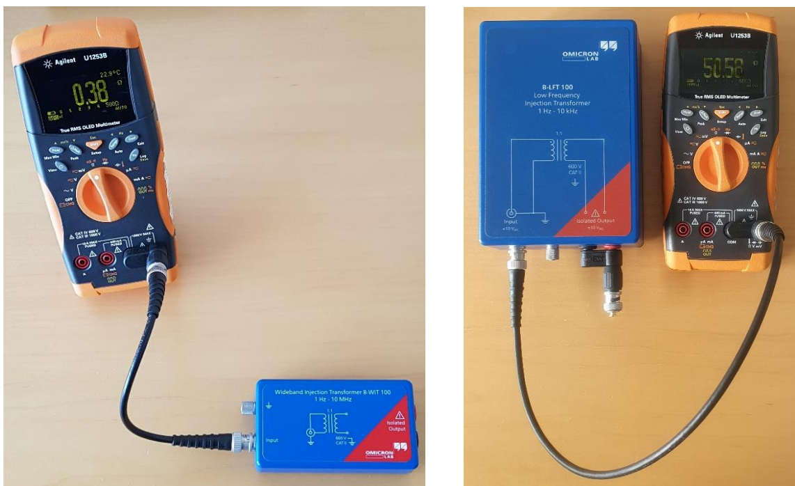
Figure 1: Measurement setup - DC resistance of input
