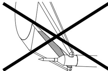
Do not grip the white plastic insulator or the probe housing with pliers.
