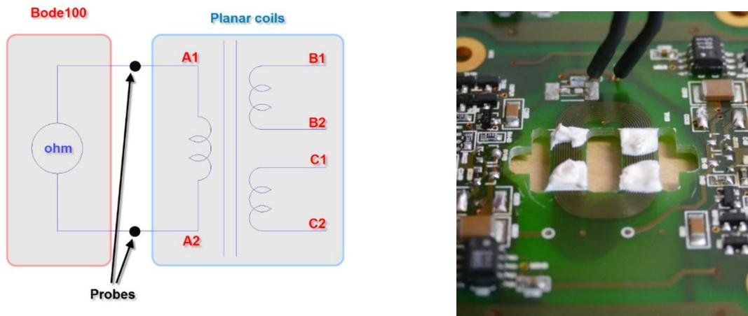
Figure 6: Outer Coil measurement setup
