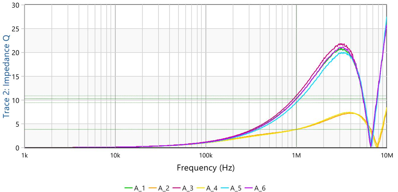
Figure 8: Outer Coil Q-Sweep
