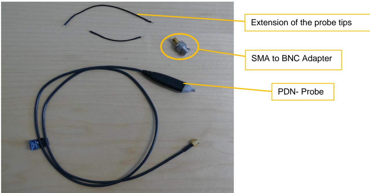
Figure 4: One-Port PDN Probe from Picotest
