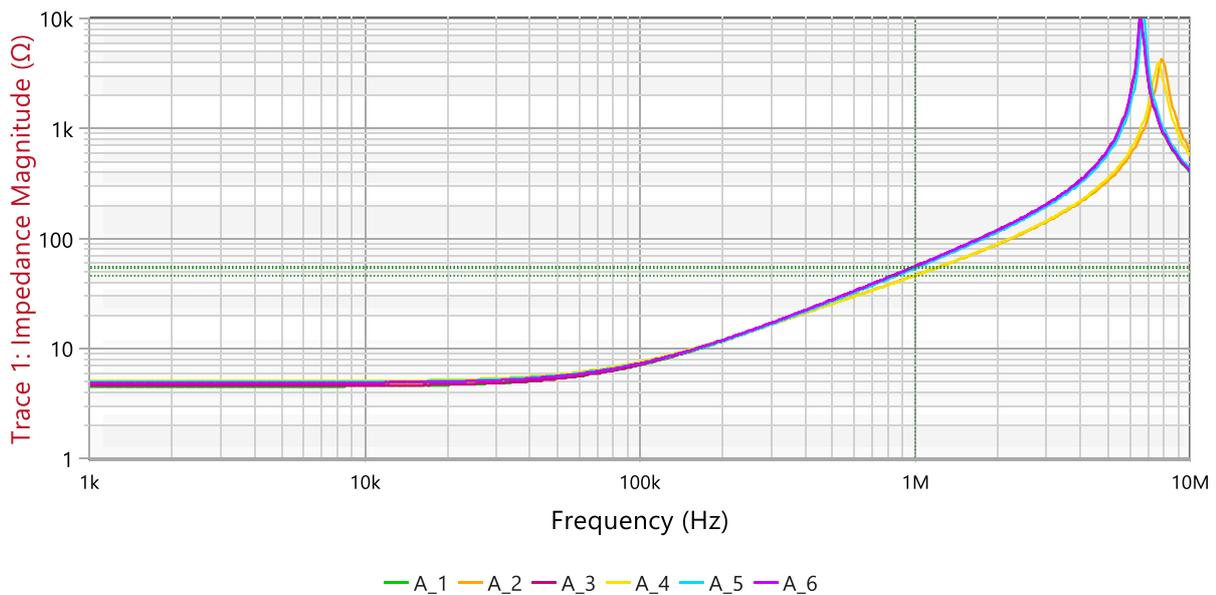
Figure 7: Outer Coil Impedance Sweep
