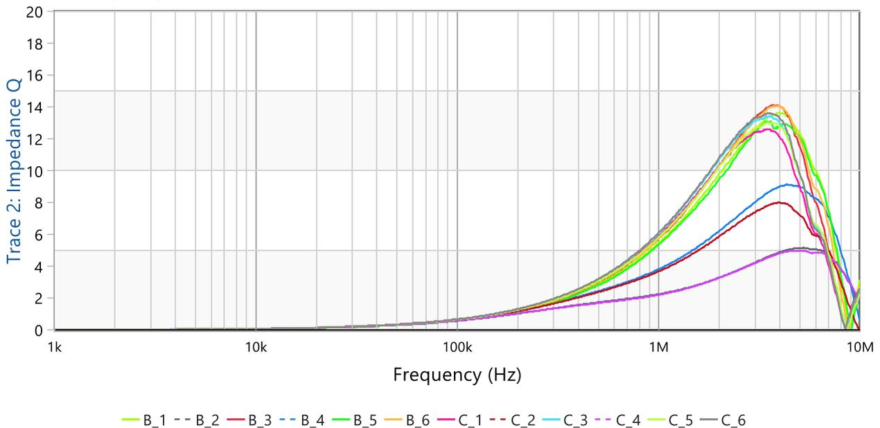
Figure 10: Inner Coil B and C, Q-Sweep
