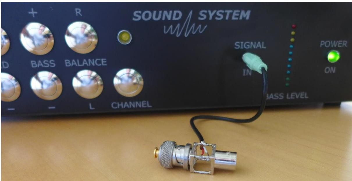
Figure 23: Output impedance measurement – sound system input
