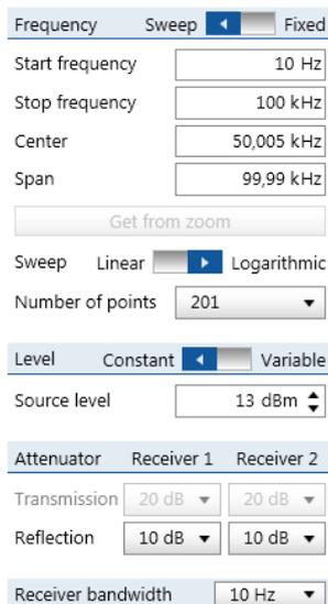
Figure 15: measurement settings – input impedance
