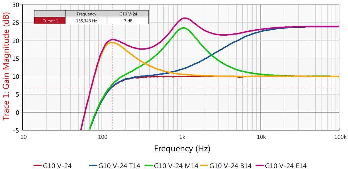
Figure 13: Gain measurement - equalizer maximum
