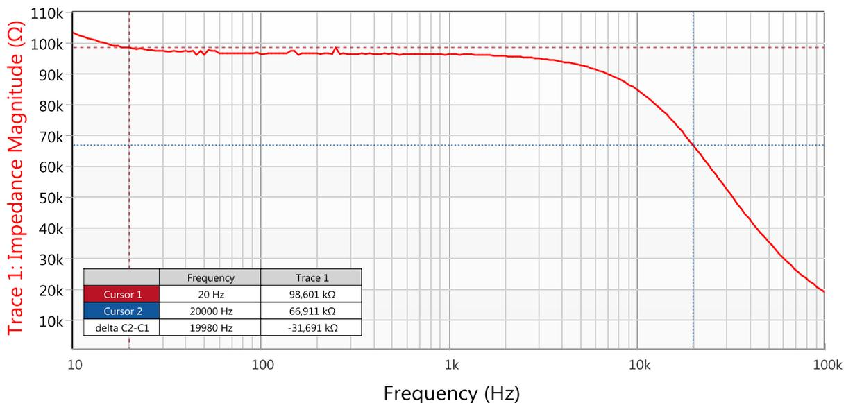
Figure 21: Input impedance with high impedance bridge - frequency sweep
