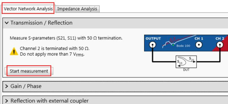
Figure 5: select measurement type transmission / reflection
