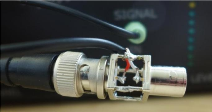
Figure 10: Audio connector to BNC connector
