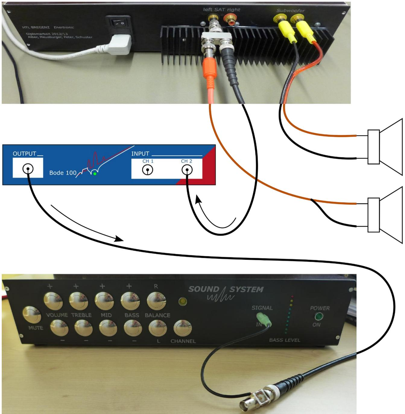
Figure 9: Gain measurement - connection setup
