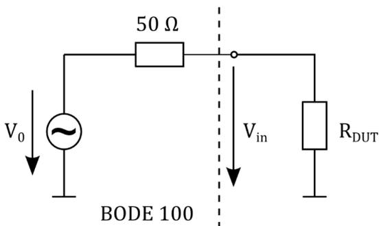
Figure 4: error estimation schematic
