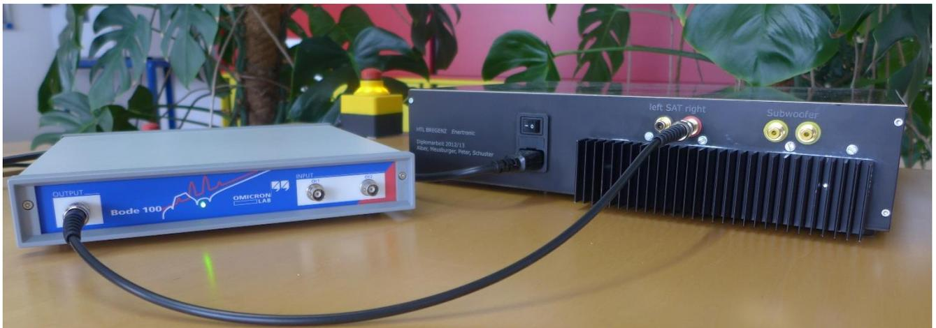
Figure 22: Output impedance measurement setup
