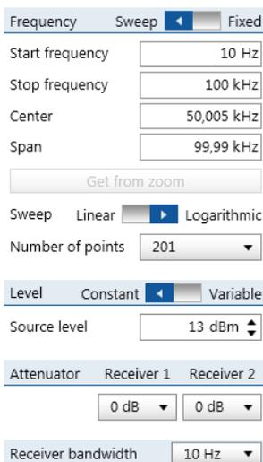
Figure 19: measurement settings external bridge
