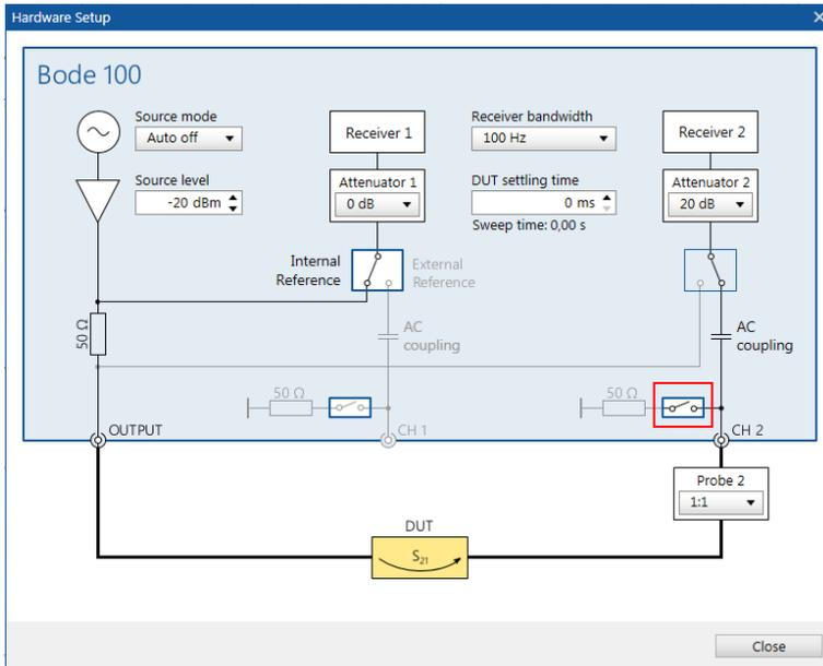
Figure 7: hardware setup window - set CH2 to 50 Ω
