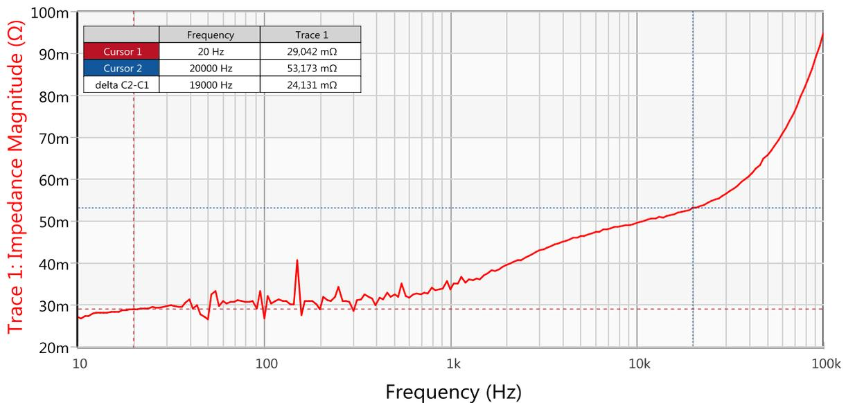
Figure 24: sound system output impedance measurement
