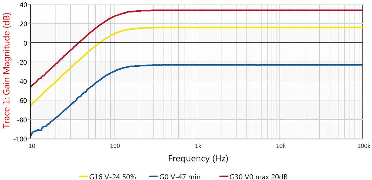
Figure 11: Gain measurement - minimum, maximum and 50 %
