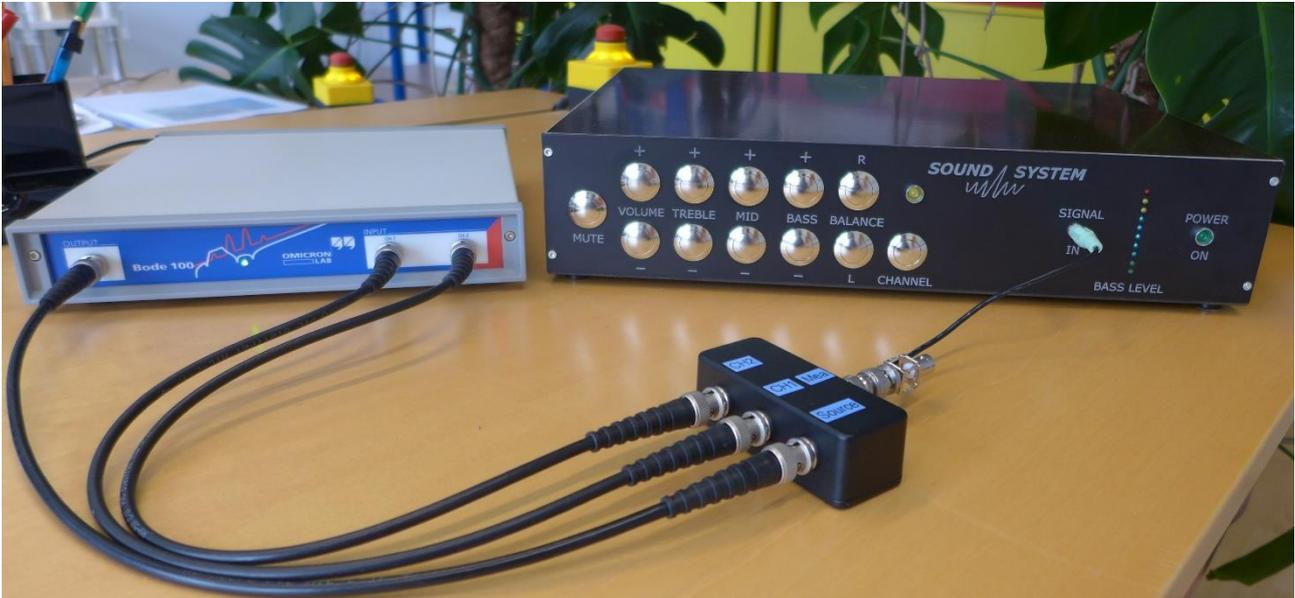
Figure 20: Input impedance with high impedance bridge - setup front view
