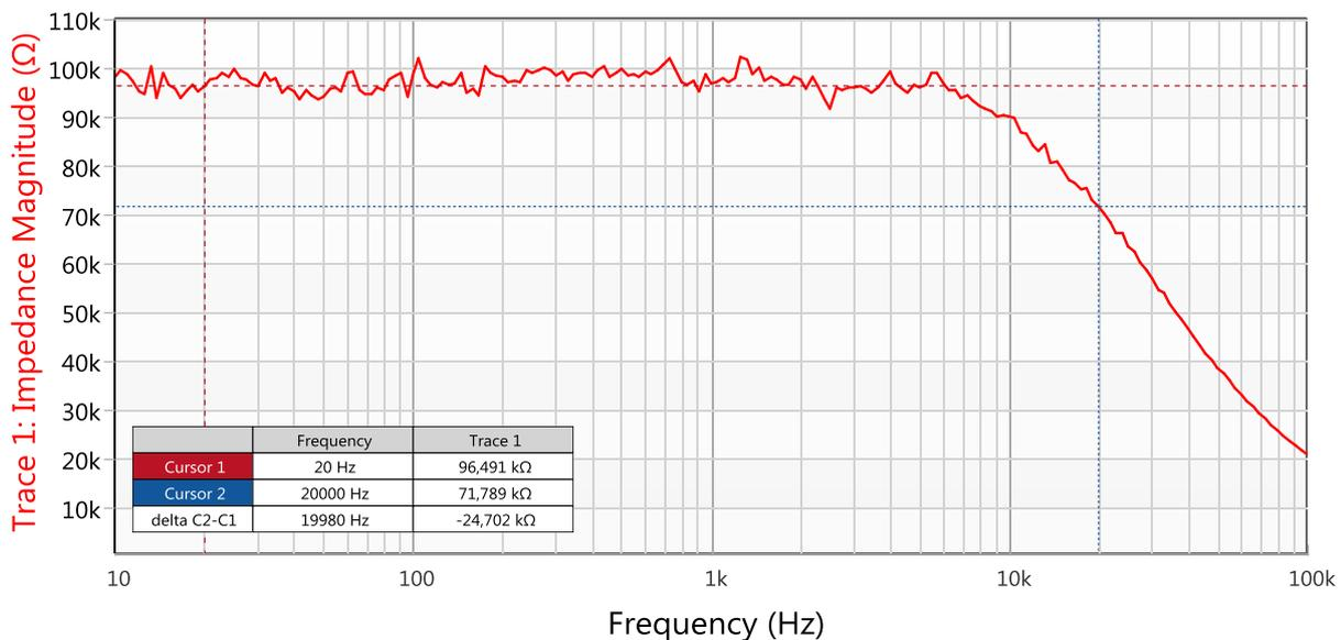
Figure 17: Standard input impedance measurement - frequency sweep
