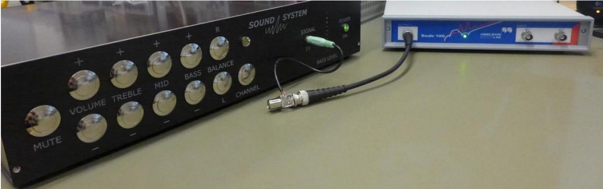
Figure 16: Standard input impedance measurement - connection setup
