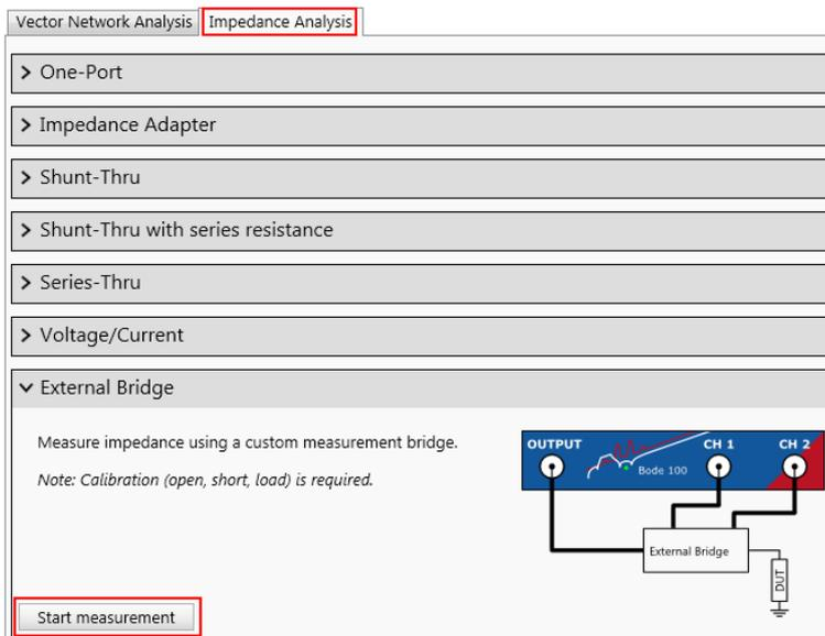
Figure 18: select measurement type external bridge
