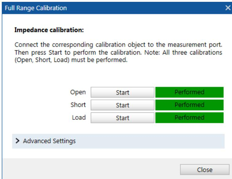
Figure 6: Probe calibration window - performed
