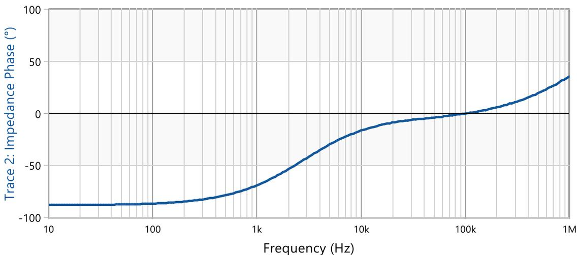
Figure 12: Phase of the impedance
