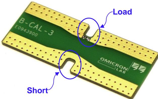
Figure 4: B-CAL calibration board
