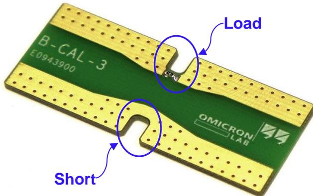
Figure 4: B-CAL calibration board
