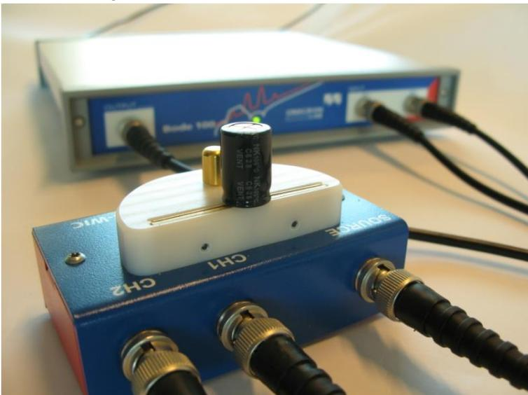
Figure 10: Capacitor connected to impedance adapter
