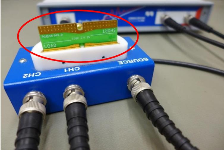
Figure 9: Impedance adapter with 100Ω load
