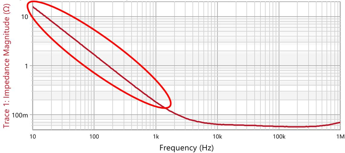
Figure 11: Frequency-dependent Impedance Magnitude
