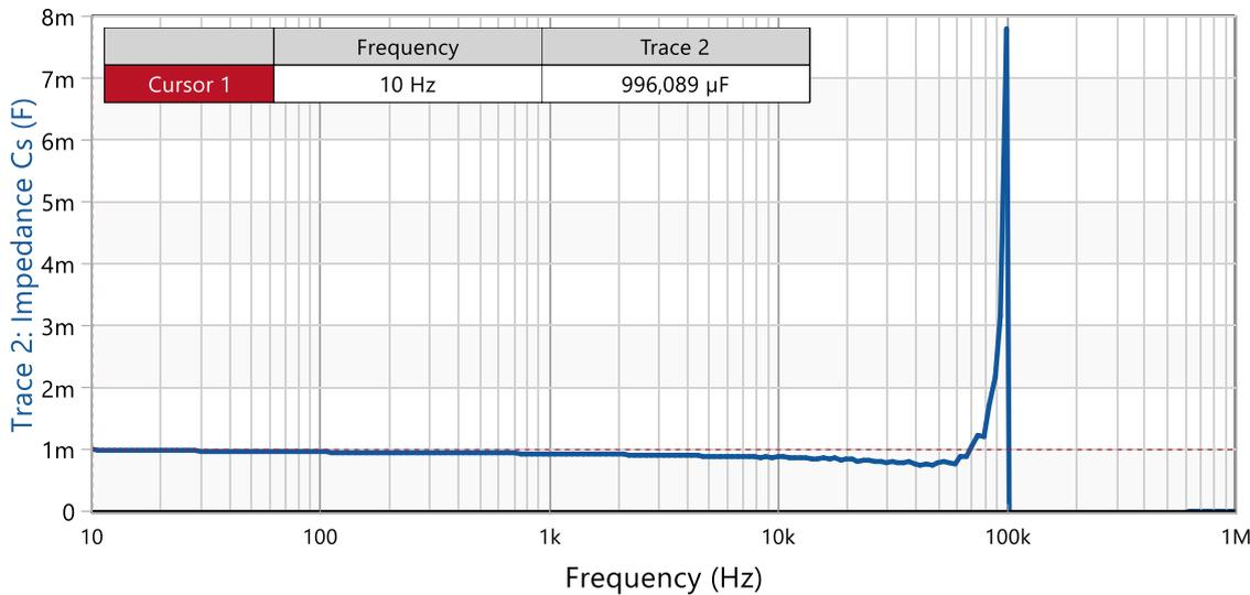
Figure 15: Series capacitance
