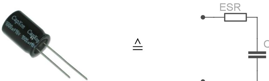
Figure 1: Capacitor equivalent circuit model
