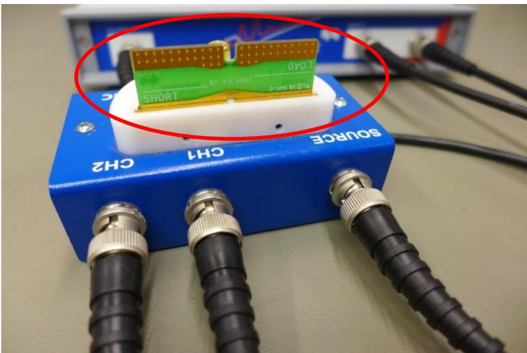
Figure 8: Short-circuited impedance adapter
