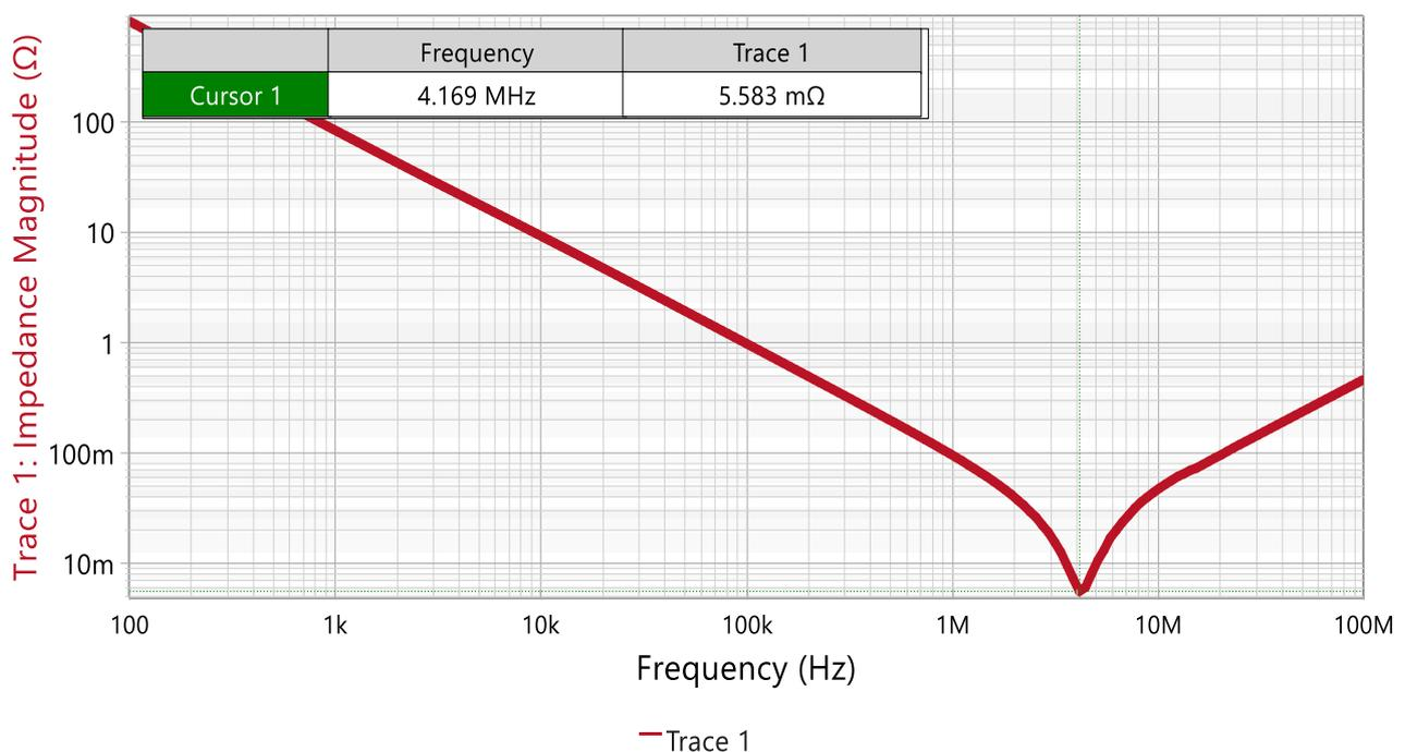
Figure 1: DUT capacitor measurement with Bode 500.
