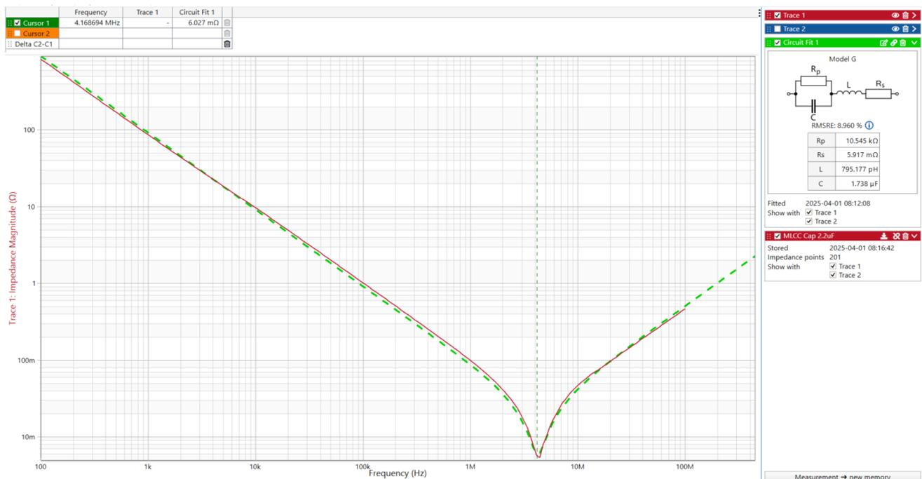
Figure 7: Circuit Fit, and measurement shown in BAS main window.
