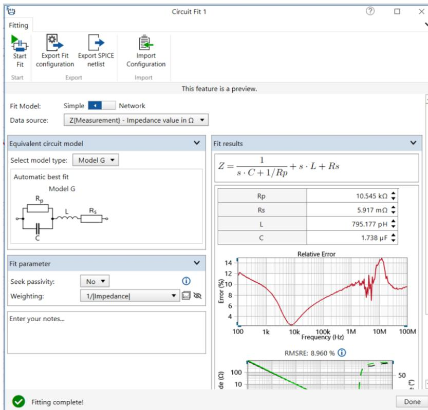
Figure 5: Circuit Fit result window.
