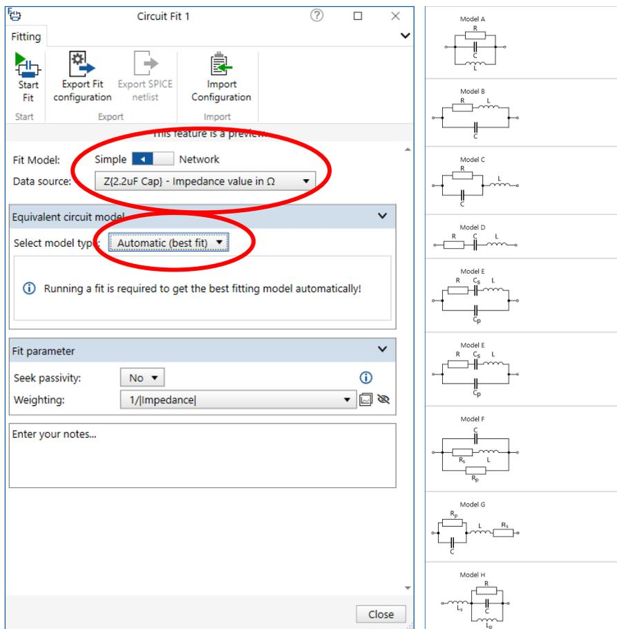
Figure 3: Circuit Fit window.
