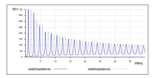
The dashed curve shows  $Re\{Z_{open}\}$  while the solid curve shows  $Re\{Z_{short}\}$
