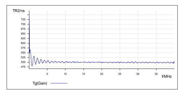
When you have a closer look at the measured curve you immediately detect a ripple. This ripple is caused by the fact that the wave impedance of the cable is not exactly 50 Ohms. The ripple amplitude increases the lower the frequency gets since the series impedance of the cable becomes more dominant at lower frequencies.
