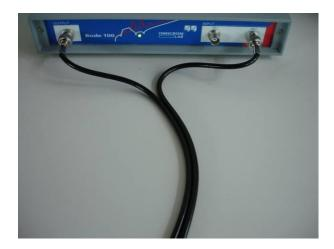
To ensure stable measurement conditions please connect a 50 Ohms load to the far end of both cables
