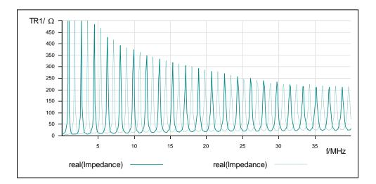
• Diagram for the measured impedance of a  $75\Omega$  cable (50 meters):
