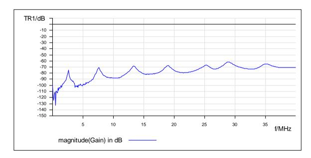
The curve shows the signal injected to our DUT (cable two). As you can see the screening is able to completely block the RF signal injected from cable one.
