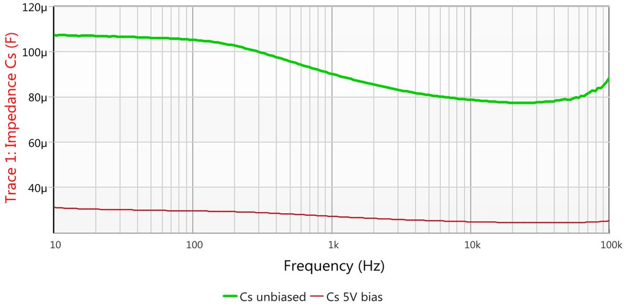
Figure 9: Trace 1 - Capacitance frequency sweep
