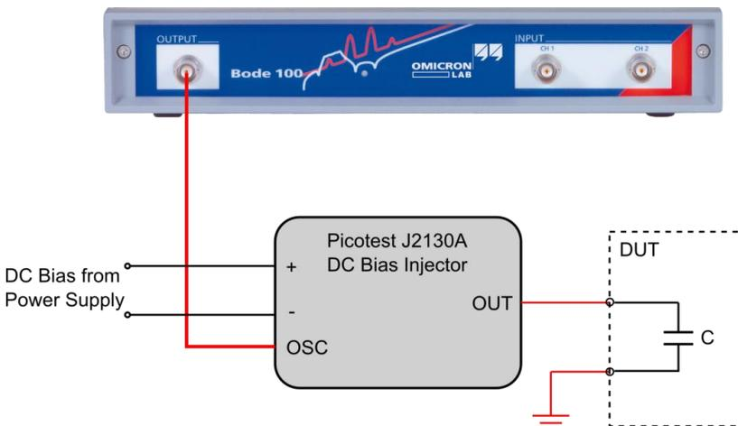
Figure 1: Capacitance Measurement Connection Diagram
