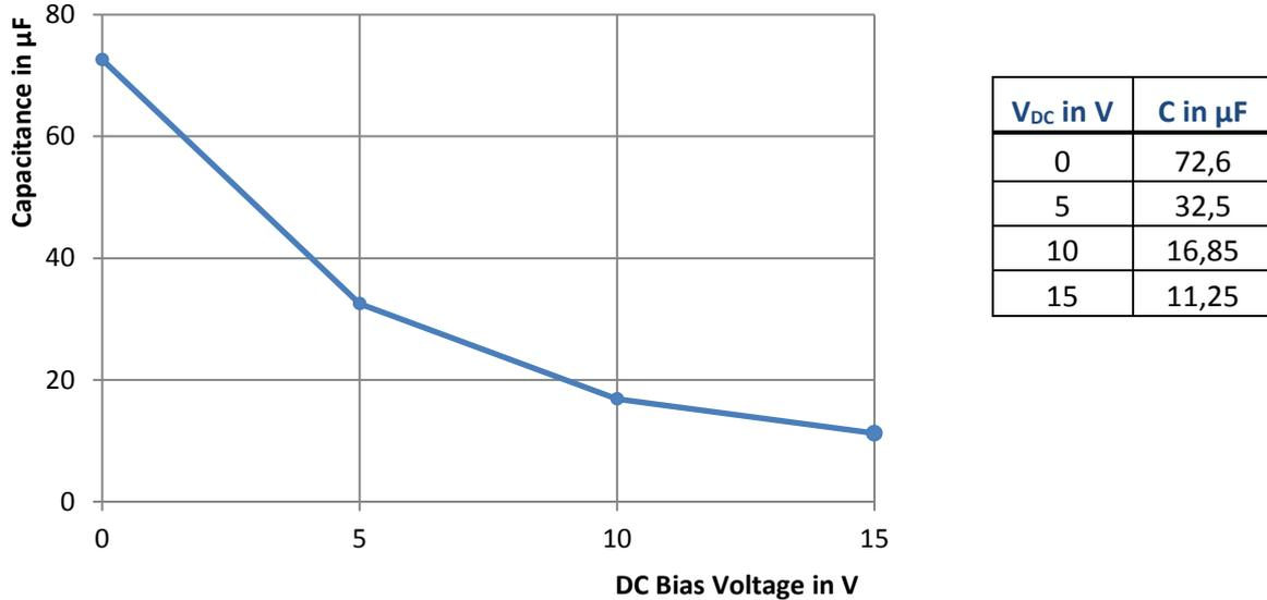
Figure 6: Change of the capacitance's with DC voltage
