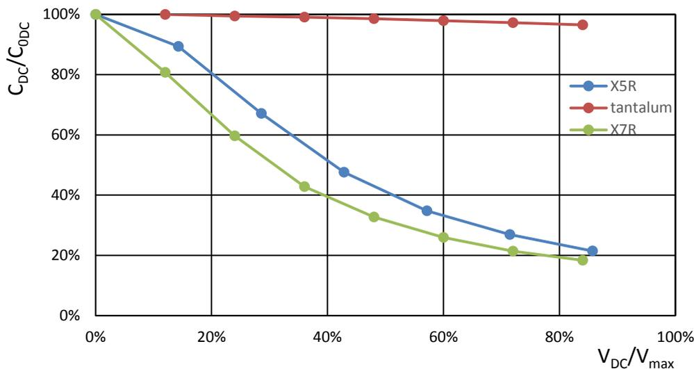
Figure 7: Comparison of the capacitance's DC voltage dependency of different capacitor types
