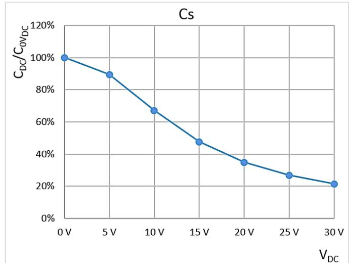
Figure 7: DC biased capacitance from datasheet.
