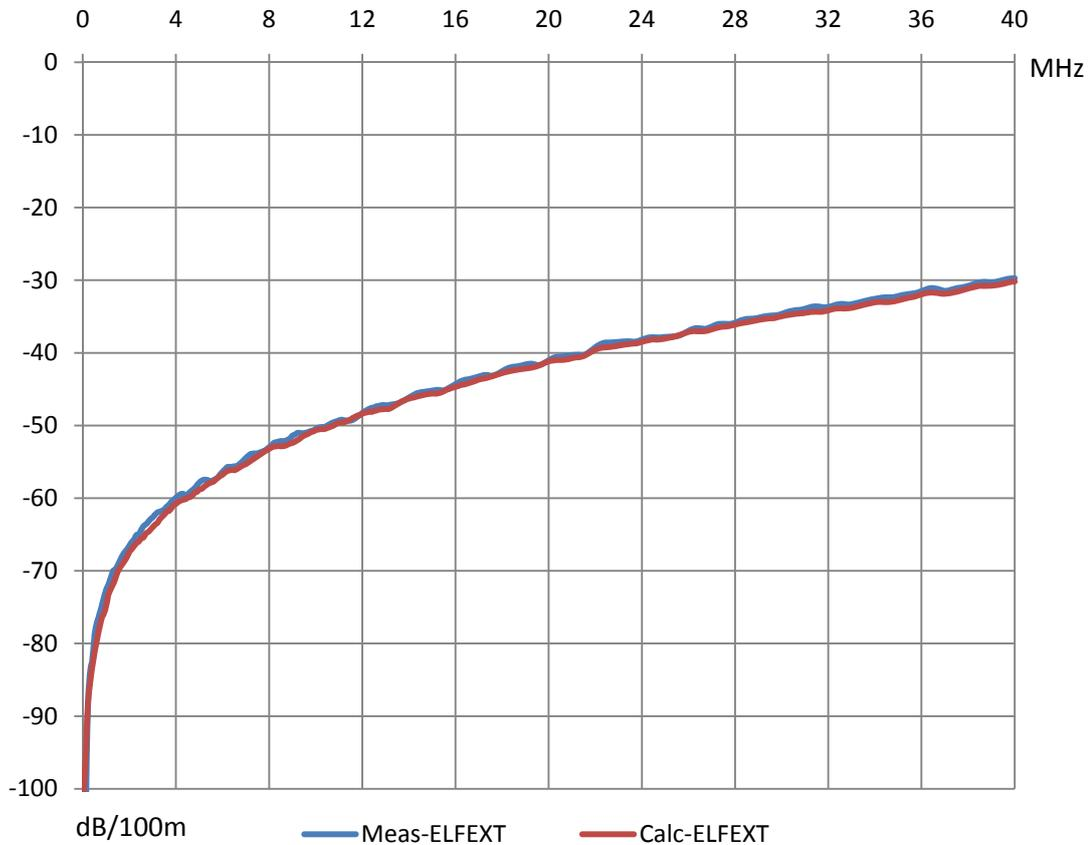
As we can see, there is no significant difference between the calculation and measurement. For that reason the direct measurement somehow is an alternative to the calculation and can be used to verify calculation results.
