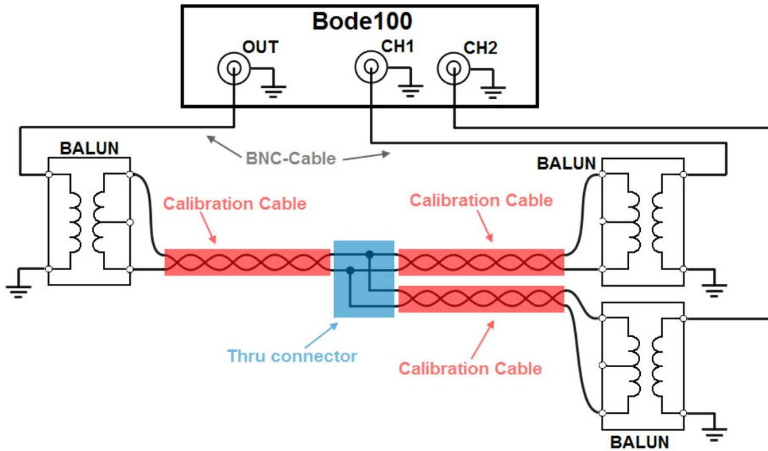
**Note:** As we can see, there is a mismatch, because two Baluns with an impedance of 50ohm are connected parallel. We are aware of this mismatch, but for the calibration we indicate, that CH1 and CH2 of the Bode 100 need the same signal level.
