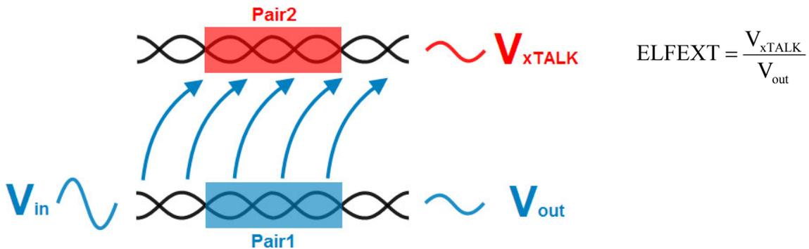
The setup for the ELFEXT measurement is almost similar to the NEXT setup. Change to the following configuration:
