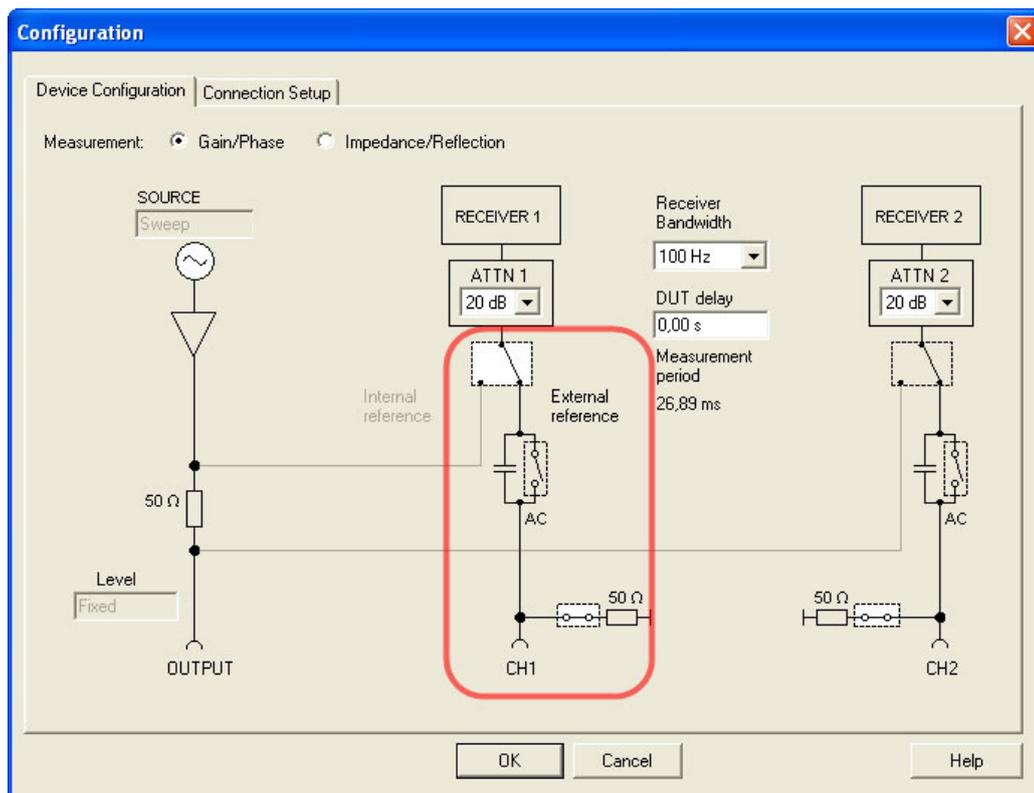
To minimize the influence of the BALUNs and cables used to connect the DUT to the Bode 100 it is advisable to perform a THRU calibration as shown in the manual in the section "Calibration in the Gain/Phase mode". Connect the Bode 100 as shown.
