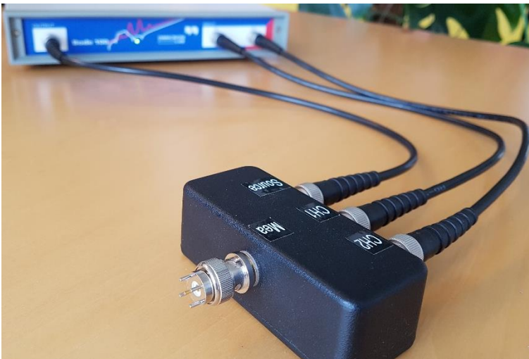
Figure 8: Open calibration with empty BNC connector
