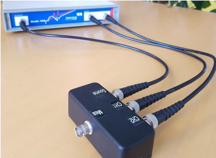
Figure 7: Open calibration nothing connected
