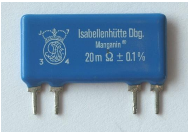
Figure 1: 20 mΩ ±0.1 % current sense resistor
