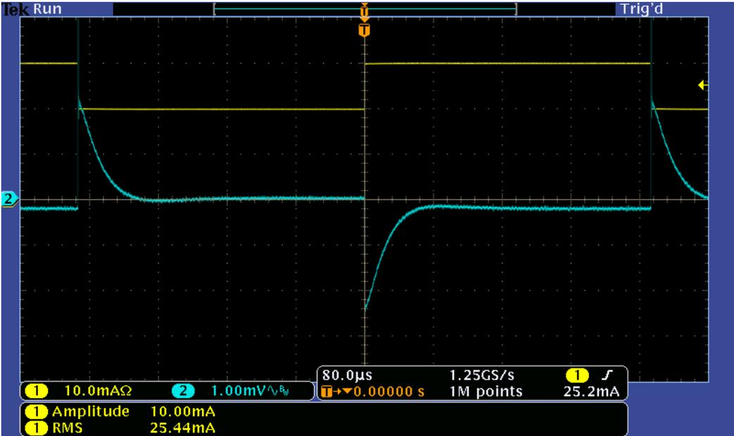
Figure 33: Step load response with aluminum capacitor.
