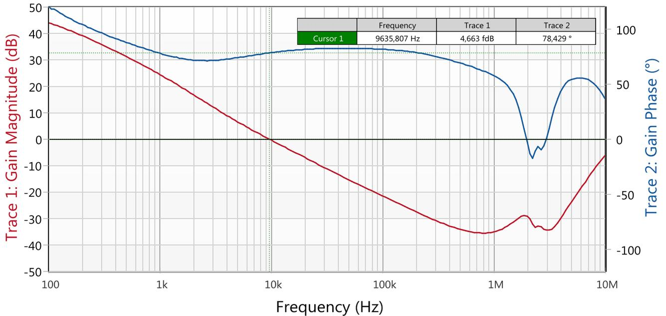
Figure 20: Bode plot with aluminum capacitor and shaped level
