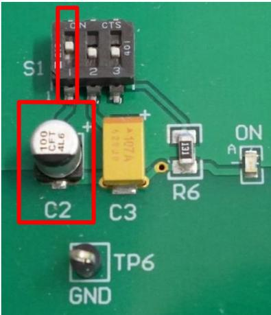
Figure 5: Capacitor C2 (aluminum)
