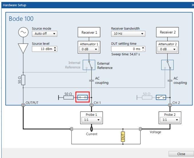
Figure 25: NISM - set CH1 to 50  $\Omega$
