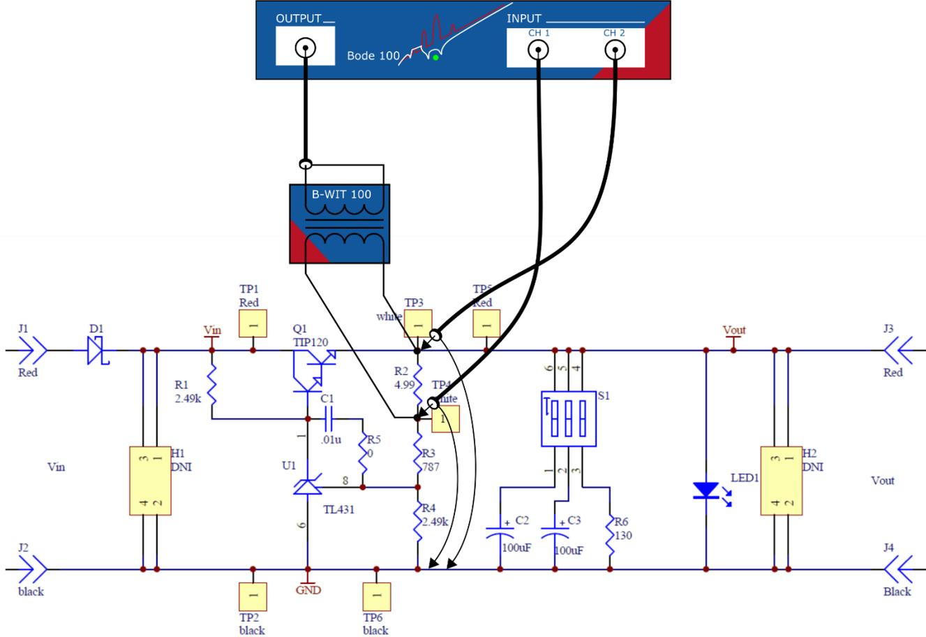
Figure 4: Schematic of the connection setup and the linear regulator
