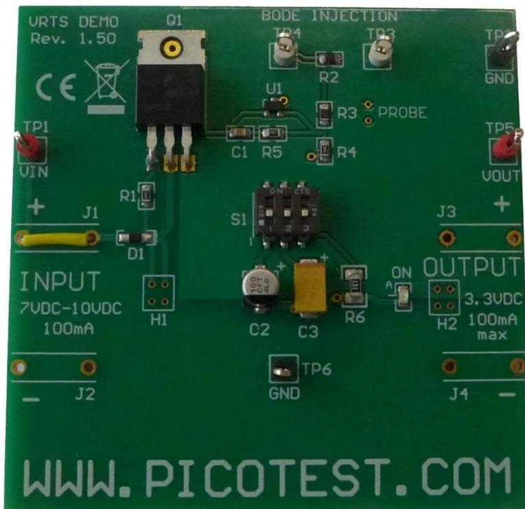
Figure 1: Voltage Regulator Test Standard board
