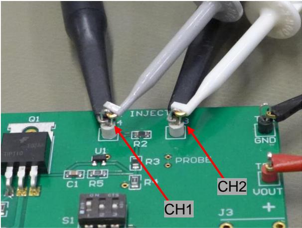
Figure 3: Connection setup of the 1:1 probes
