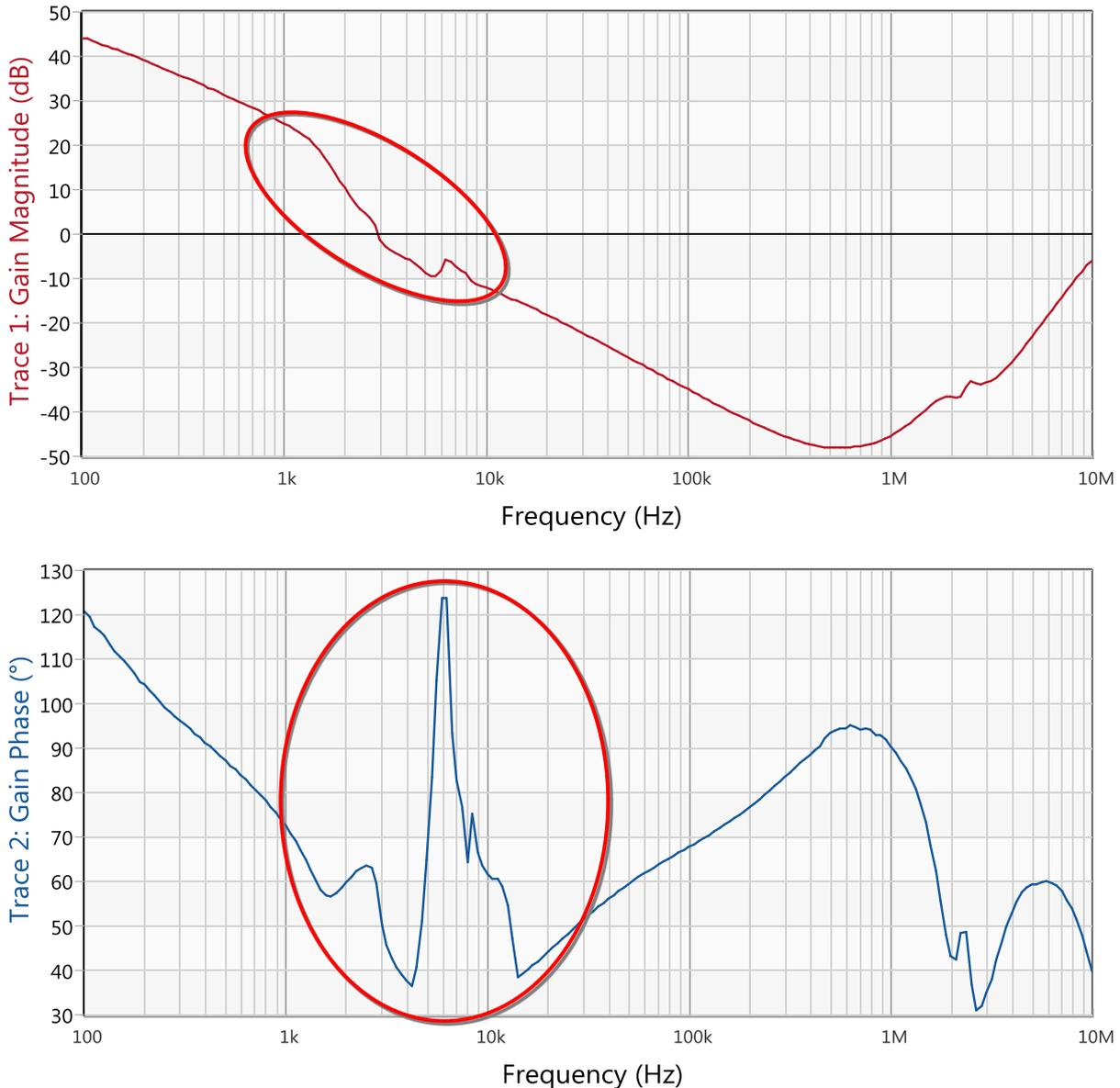
Figure 15: Bode plot with tantalum capacitor and 0 dBm output power level
