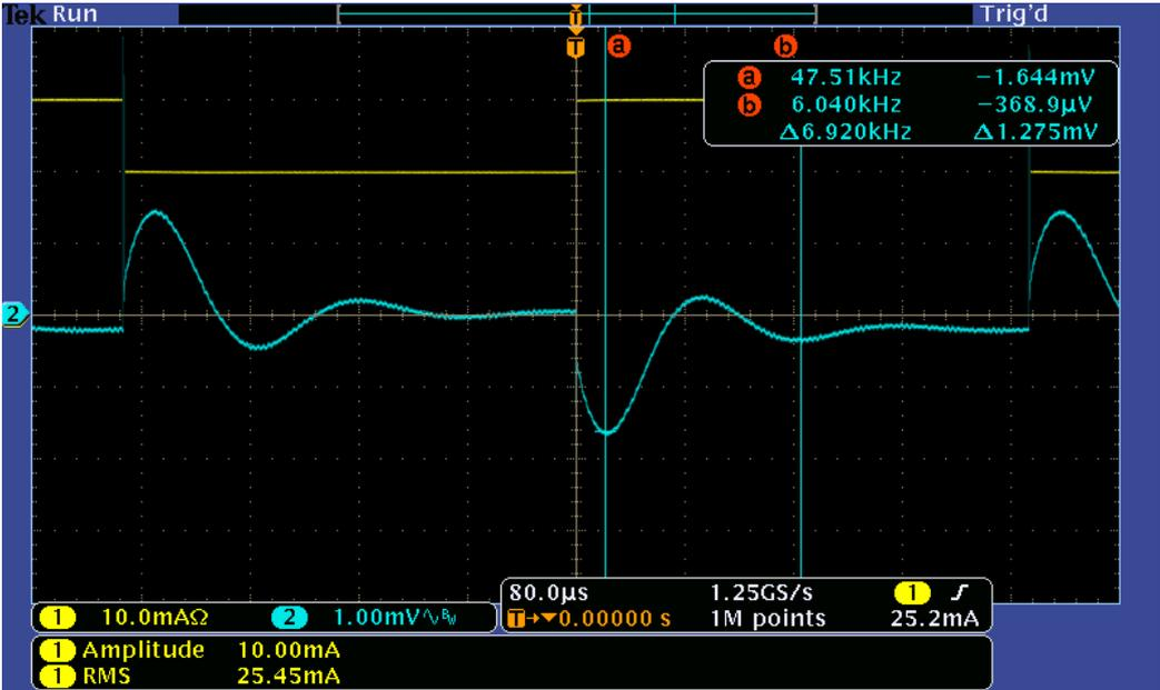
Figure 32: Step load response with tantalum capacitor
