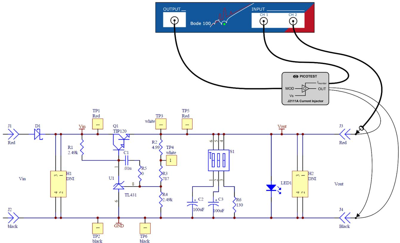
Figure 21: Output impedance measurement using Bode 100 and Picotest J2111A
