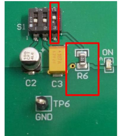
Figure 7: Resistor R6 (load)
