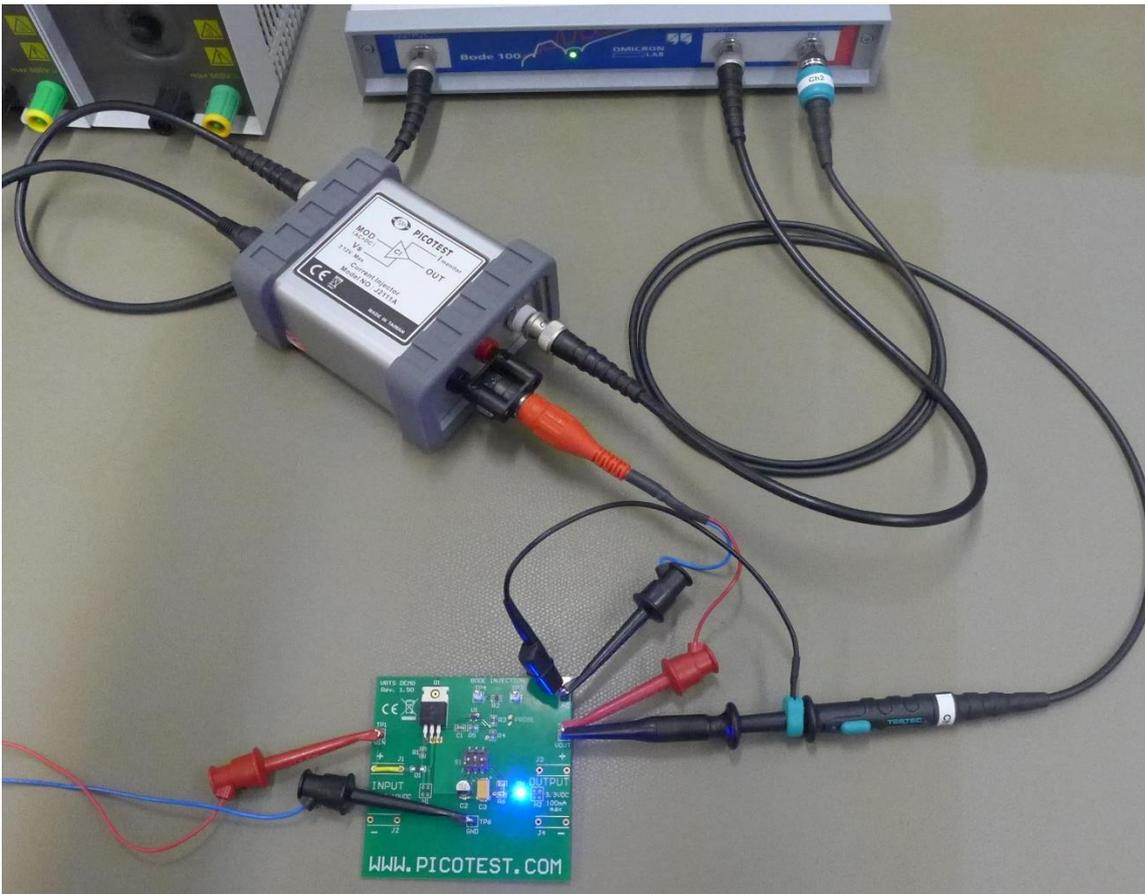
Figure 22: Output impedance measurement example
