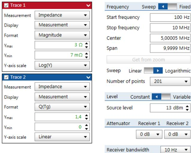
Figure 26: NISM - Trace and measurement settings
