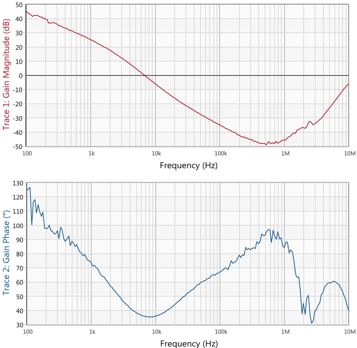
Figure 16: Bode plot with tantalum capacitor and  $-27$  dBm output level
