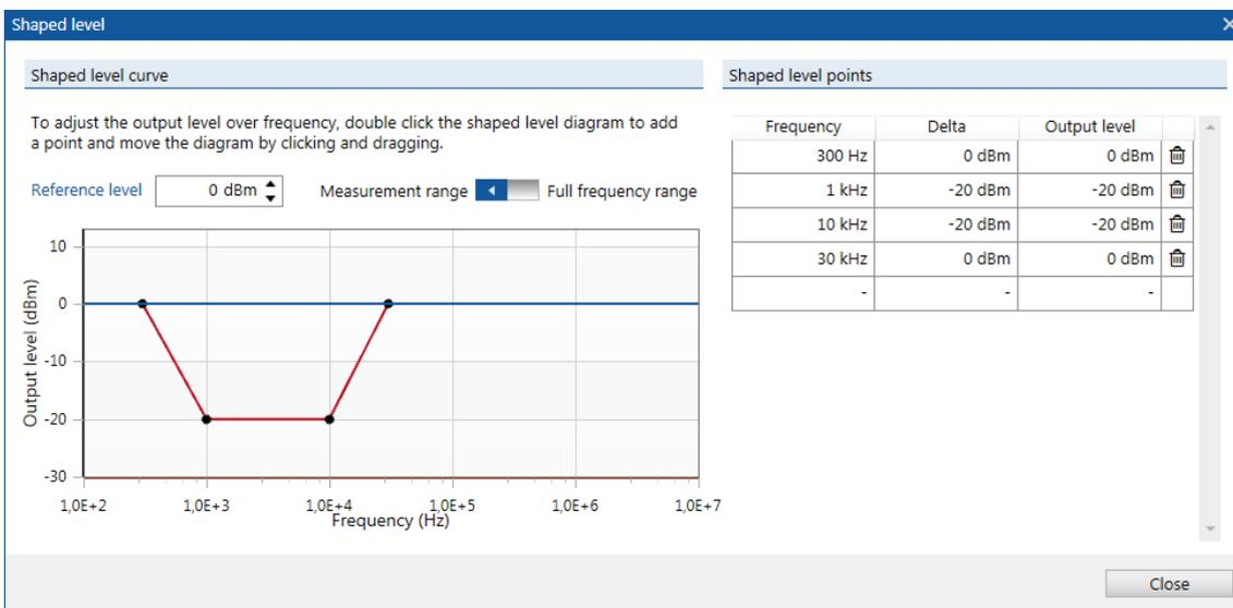
Figure 18: Shaped level window
