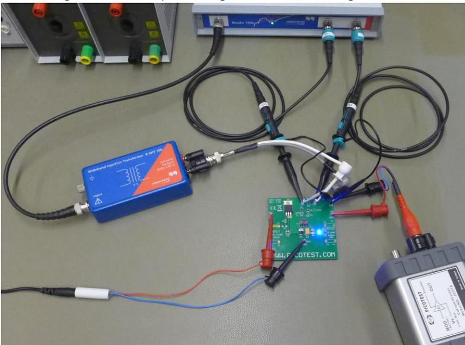
Figure 2: Loop Gain measurement setup with Bode and B-WIT
