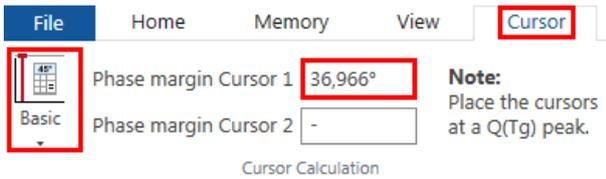
Figure 27: NISM - basic phase margin calculation
