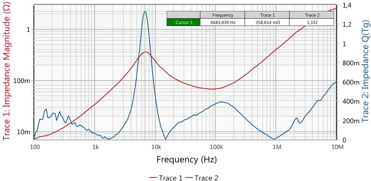
Figure 28: Output impedance with tantalum capacitor
