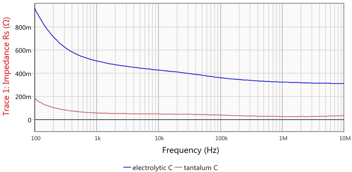
Figure 31: ESR measurement of C2 and C3
