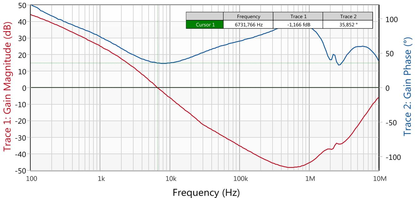
Figure 19: Bode plot with tantalum capacitor and shaped level
