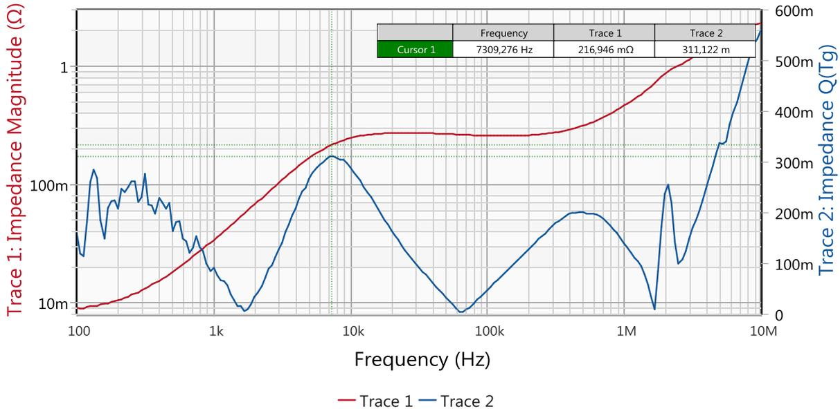
Figure 29: Output impedance with aluminum capacitor
