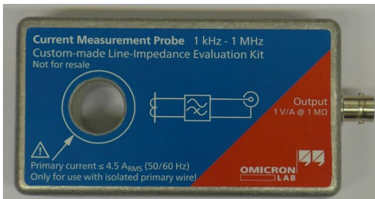
Figure 2: Custom-made current measurement probe
