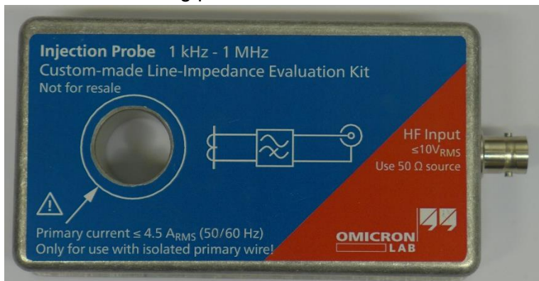
Figure 1: Custom-made injection probe
