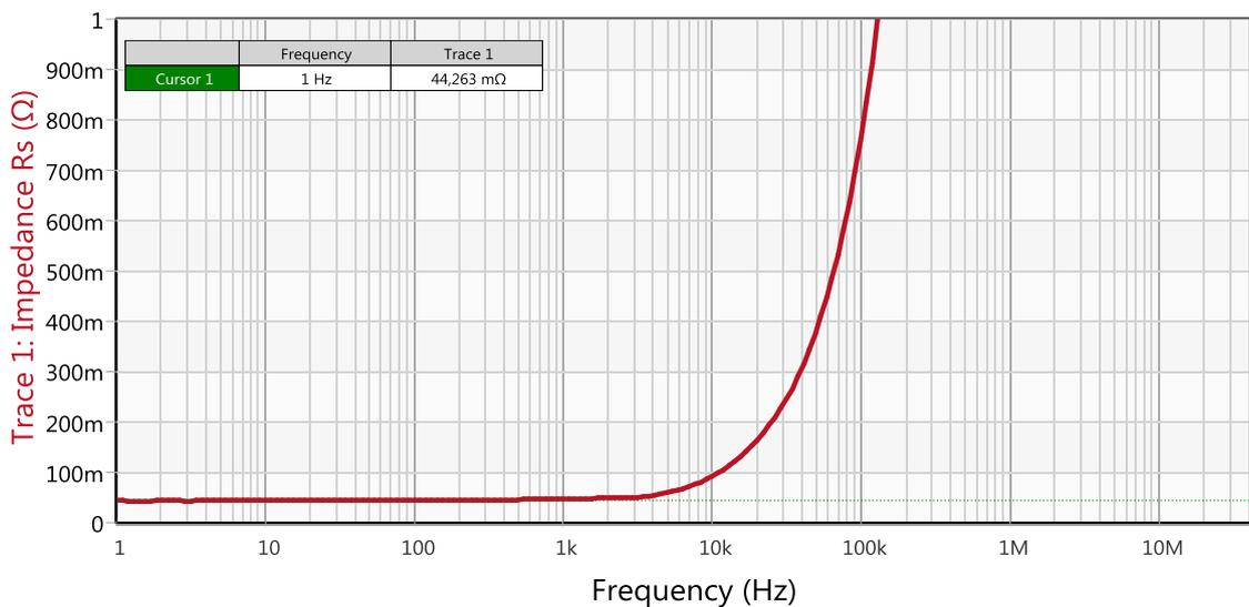
Figure 11: Measurement result – series resistance
