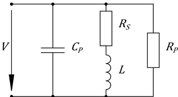
Figure 2: Circuit model with parasitic elements
