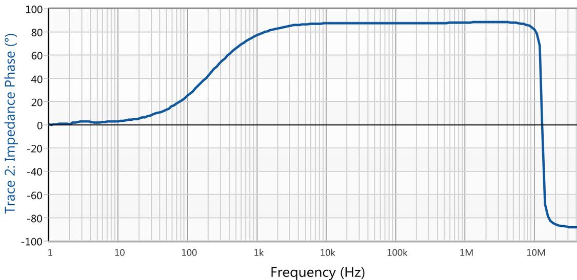
Figure 9: Measurement result - Phase ( $^\circ$ )
