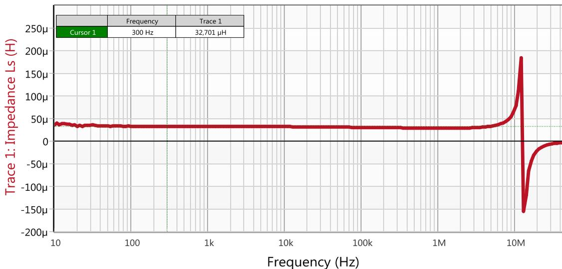
Figure 13: Measurement result - inductance
