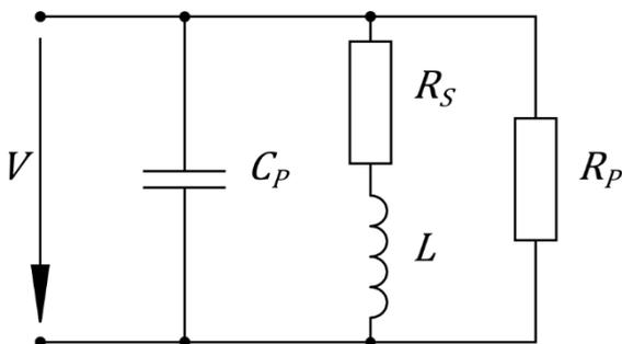
Figure 2: Circuit model with parasitic elements
