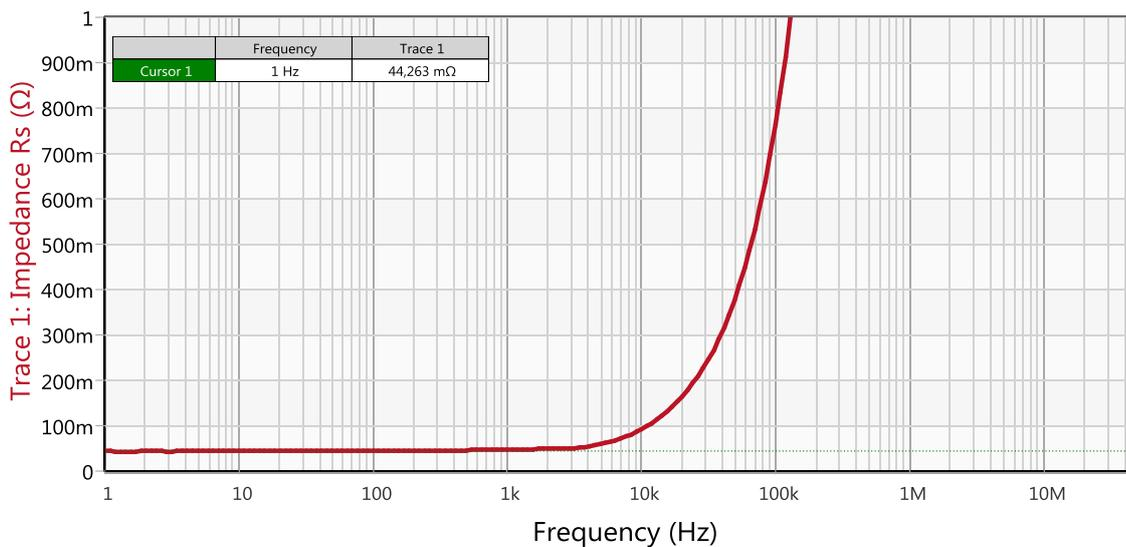
Figure 11: Measurement result – series resistance
