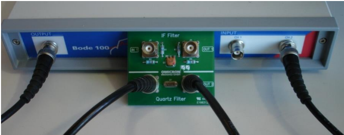
Figure 8: Setup with quartz filter
