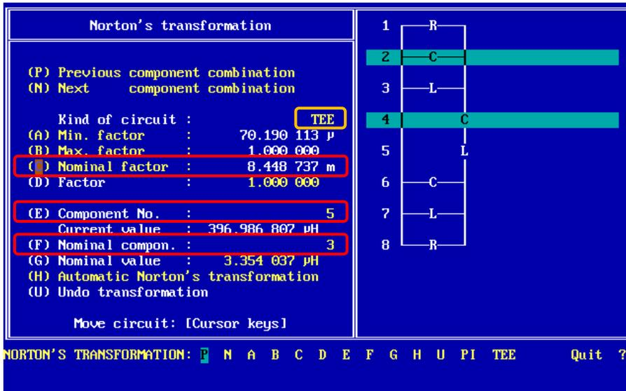
In addition the <Kind of circuit> is set to TEE as this gives a better structure for the second transformation.
