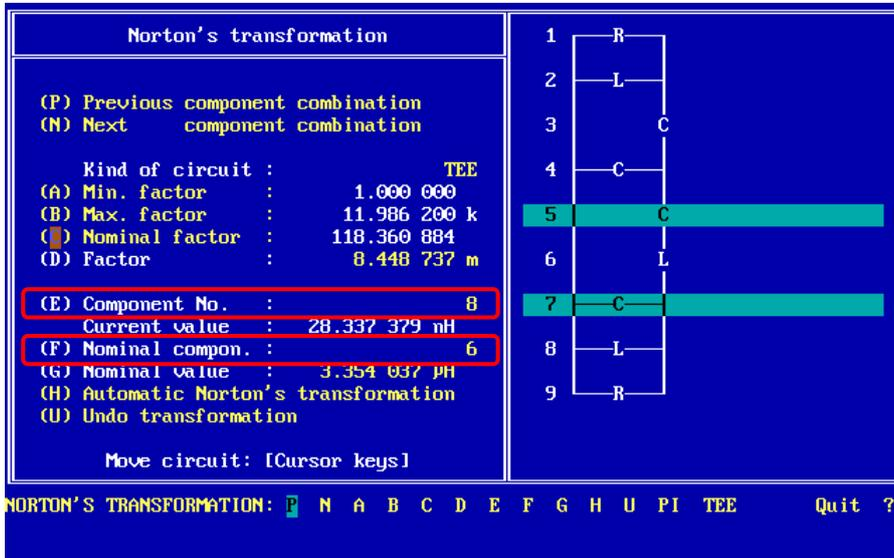
Performing the transformation by clicking on <Nominal factor> leads to the final circuit design. The circuit and component values can be displayed by clicking on <Quit> and <Output circuit>:
