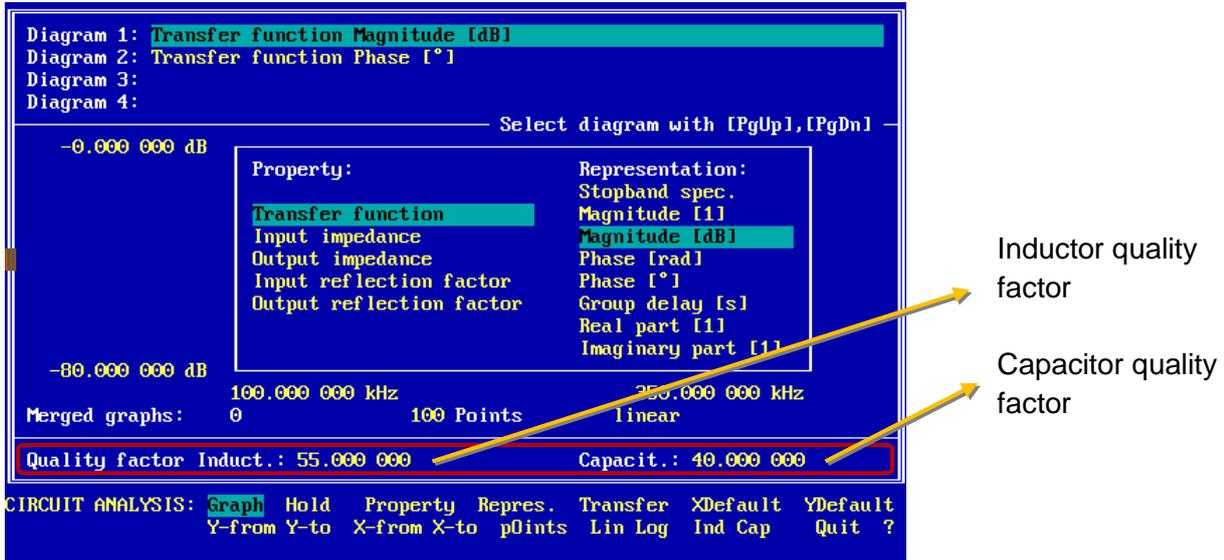
When considering the quality factors of the components the calculated transfer characteristic results as shown in the following graph:
