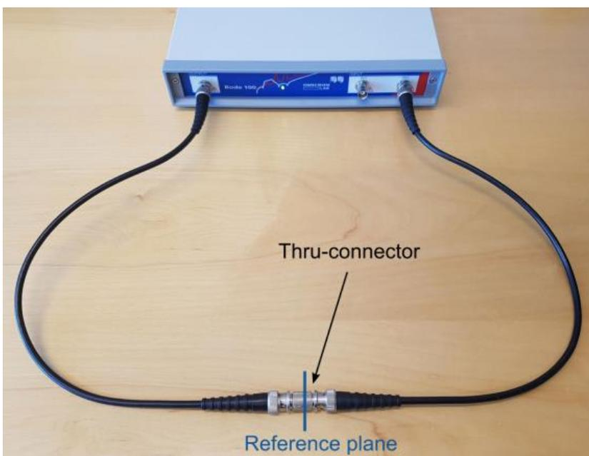
Figure 5: Calibration setup
