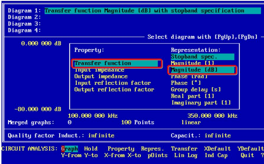
Clicking on <Graph> starts the plot window and shows the transfer function as shown in the following figure.
