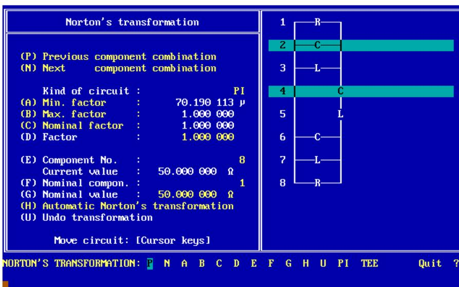
The transformation always works from top to down. We now want to perform a transformation in a way that the inductor L5 gets the same inductance value as the inductor L3. This can be done by setting the <Component No.> to 5. This means that component No. 5 will be changed. Since we want the inductor L5 to have the same value as the inductor L3 the <Nominal compon.> has to be set to 3. QuickFil now calculates the transformation factor which is displayed in the <Nominal factor> field:
