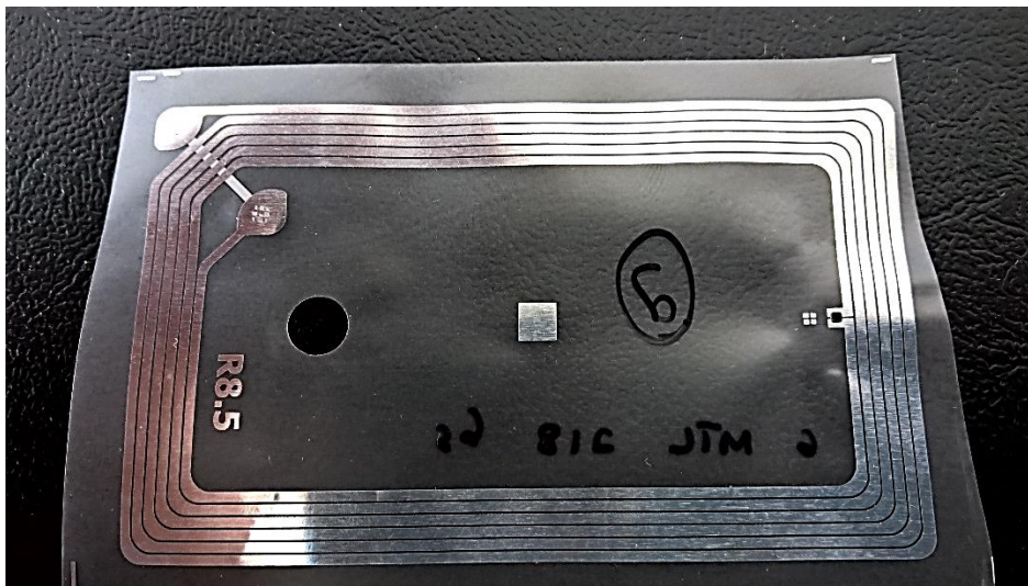
Figure 11: Transparent Foil with RFID Antenna and Chip
