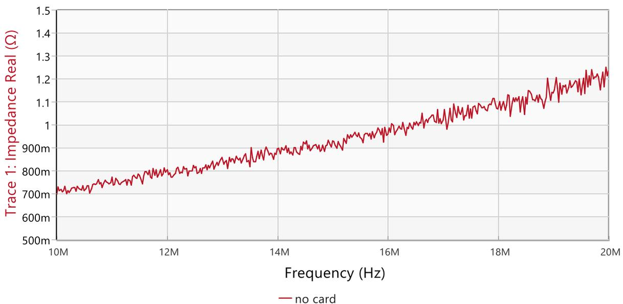
Figure 8: Series Resistance of B-RFID-A Coupling Coil
