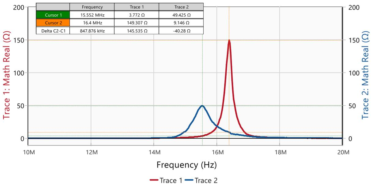
Figure 11: Resonance Frequency Measurement
