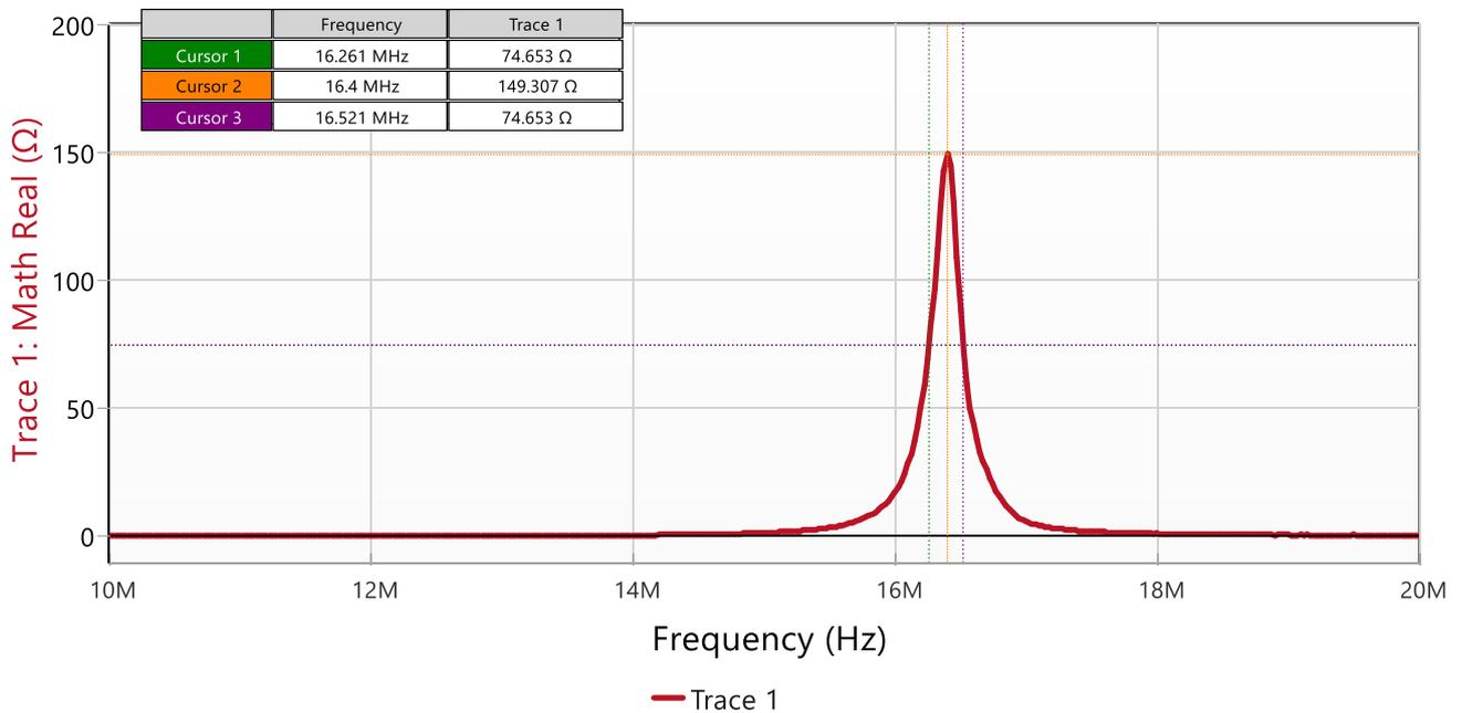
Figure 14: measurement curve and cursors for Q measurement
