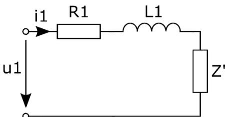
Figure 4: Transformed Equivalent Circuit
