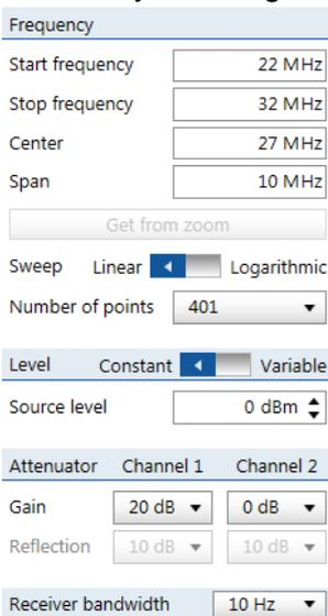
Figure 16: Settings for the measurement
