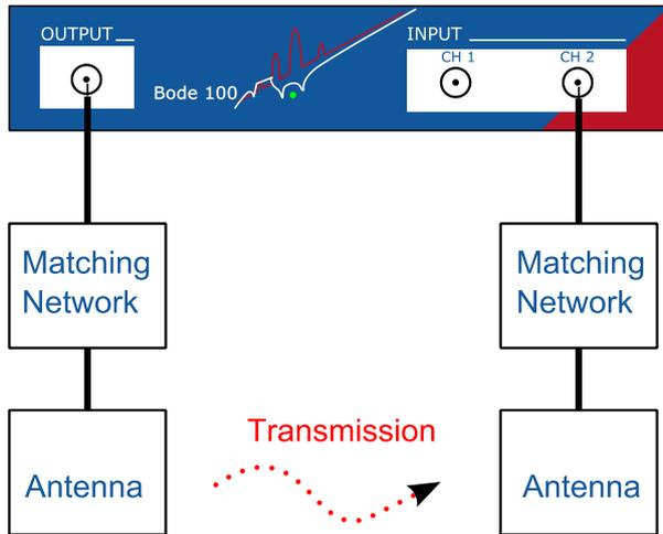
Figure 15: Picture of the following setup
