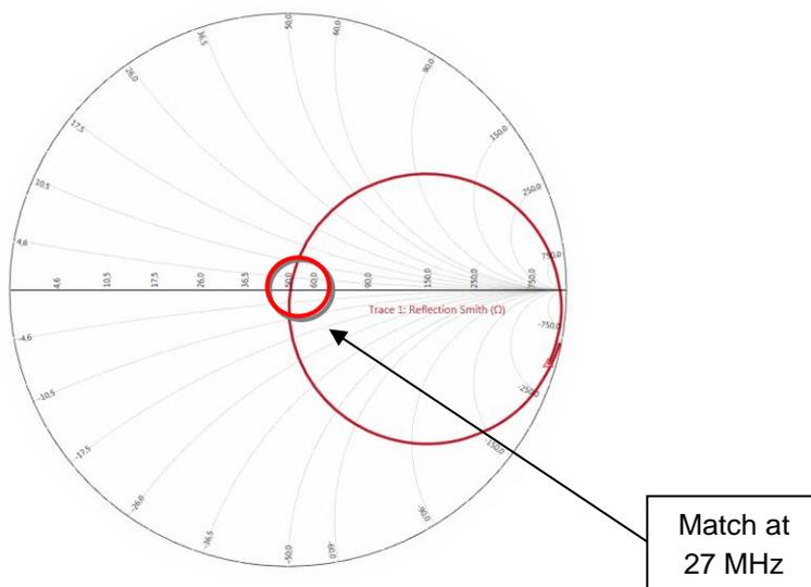
Figure 14: Impedance with matching network
