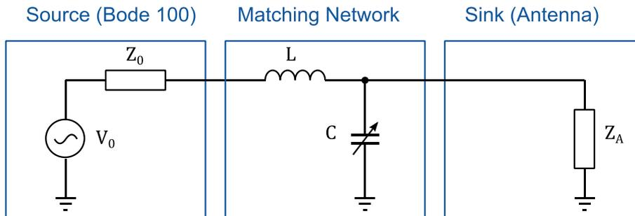
Figure 10: Network with a matching network
