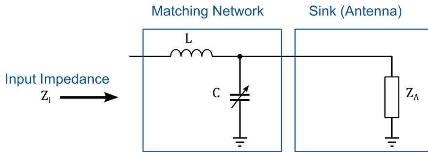
Figure 11: Network for measuring the Input Impedance
