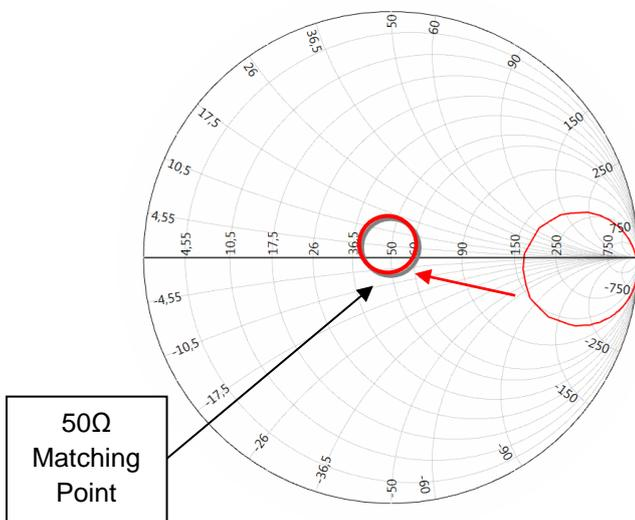
Figure 13: Impedance without matching network
