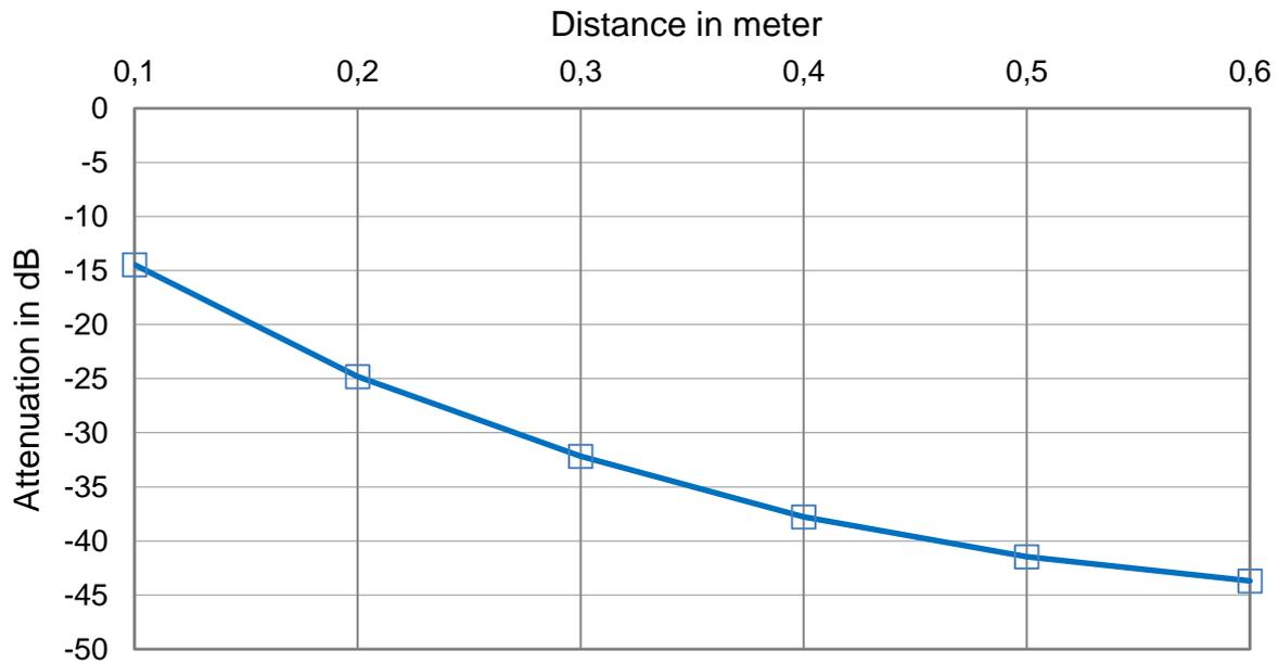
Figure 21: Attenuation to Distance curve
