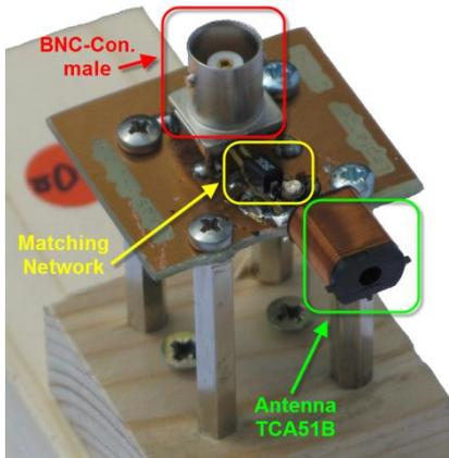
Figure 2: Antenna setup
