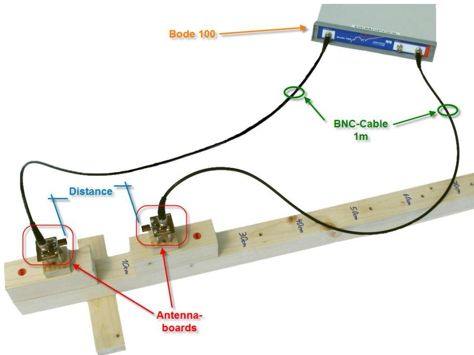
Figure 18: Measurement setup
