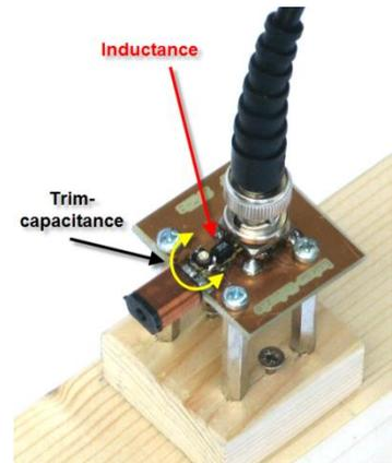
Figure 12: Setup of the antenna
