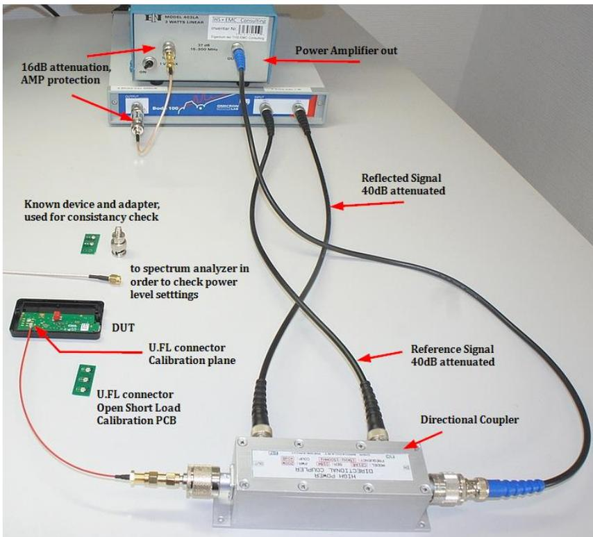
Figure 4: Measurement setup
