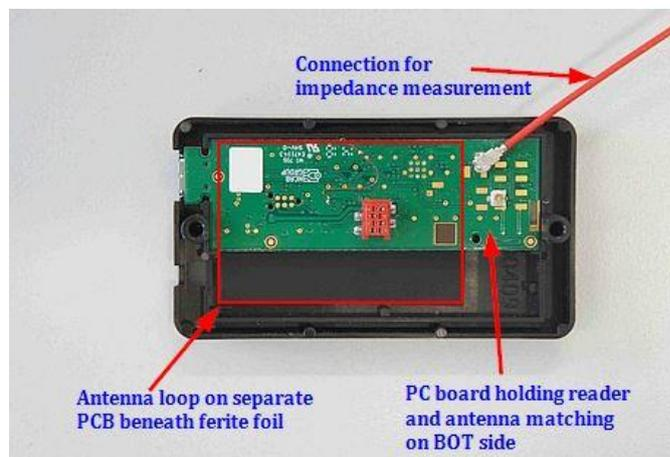
Figure 1: RFID Reader DUT
