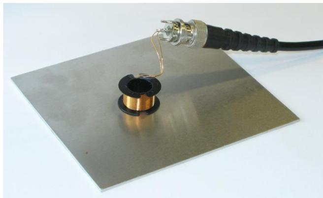
Figure 8: eddy current measurement
