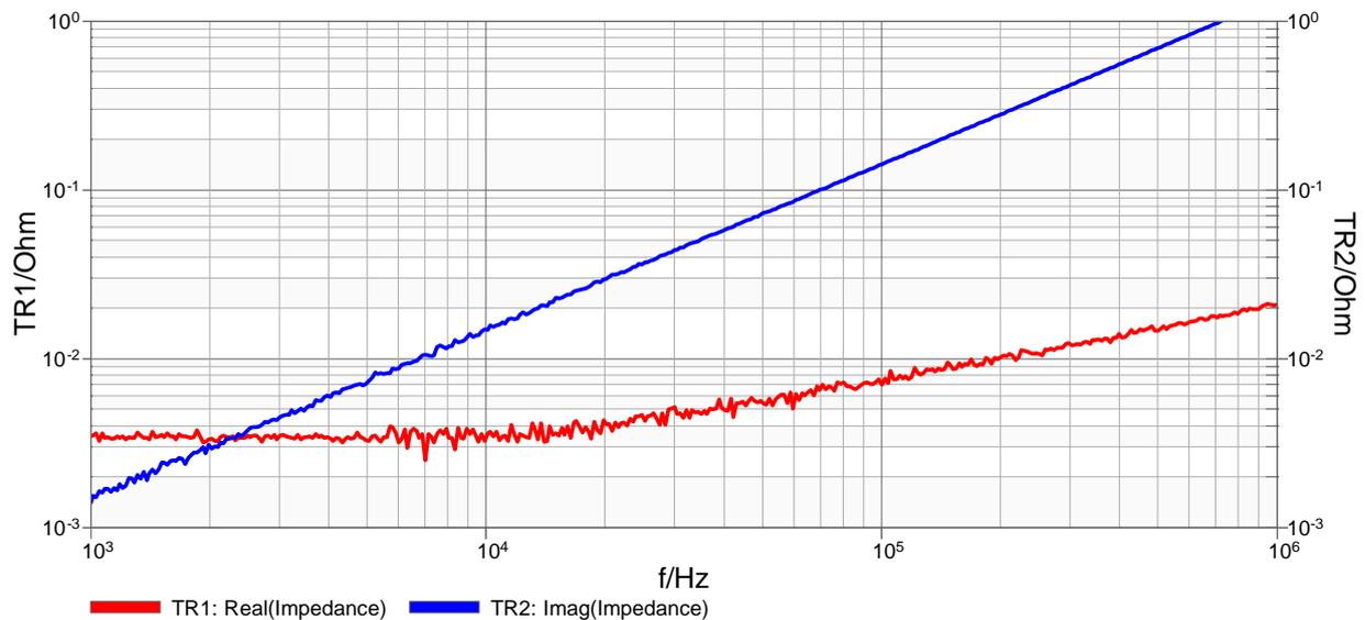
Figure A6: inductance and resistance measurement
