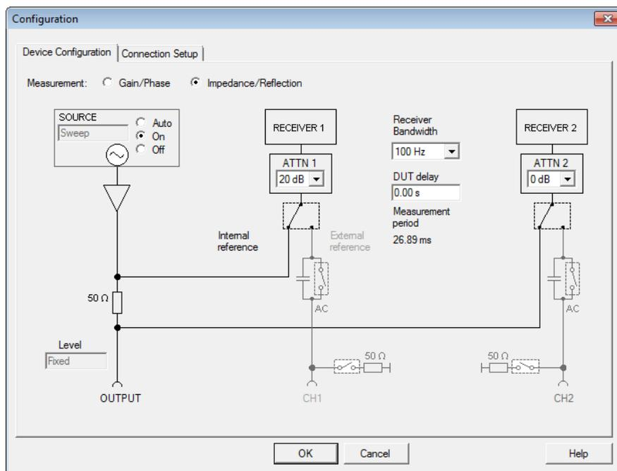
Figure 1: internal configuration of the Bode 100
