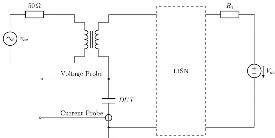
Figure 2.3: Dc biased impedance measurement circuit with inductive decoupling of the ac source
