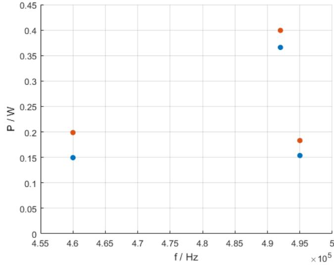
Figure 6.20: Measured and calculated losses of the output capacitor for the three measurement points. Blue: measured losses; red: calculated losses
