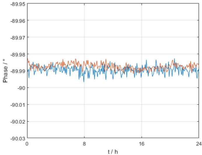
Figure 4.12: Phase of the C0G capacitor over time. Blue: measurement bridge; red: TCM
