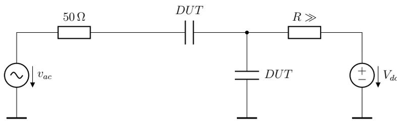
Figure 2.4: Dc biased impedance measurement circuit using two equal capacitors
