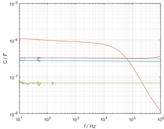
Figure 5.1: Capacitance of capacitors versus frequency without dc bias. Blue: CeraLink; red: e-cap; yellow: X7R; violet: film; green: C0G
