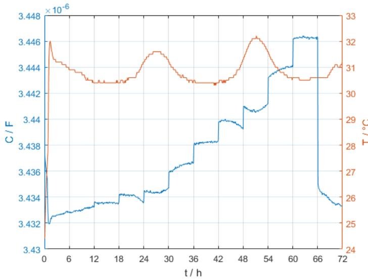
Figure 4.3: Capacitance change over voltage and time. Blue: capacitance; red: ambient temperature
