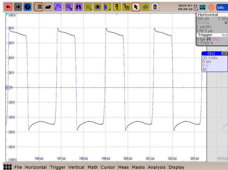
Figure 6.14: Measured inductor voltage at 460 kHz
