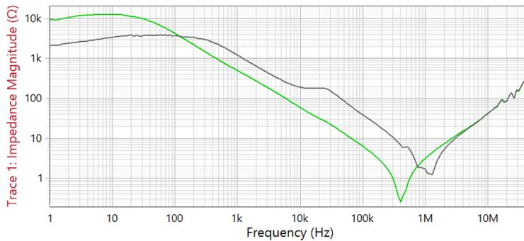
Figure 3.2: Output impedance of the used voltage source at 50 V (green) and 1000 V (grey)
