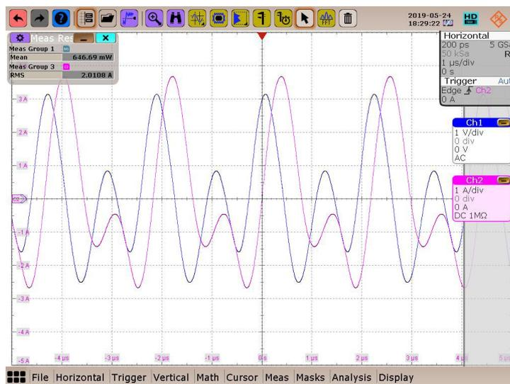
Figure 6.11: Ac voltage (blue) and current (pink) of the output capacitor at 460 kHz
