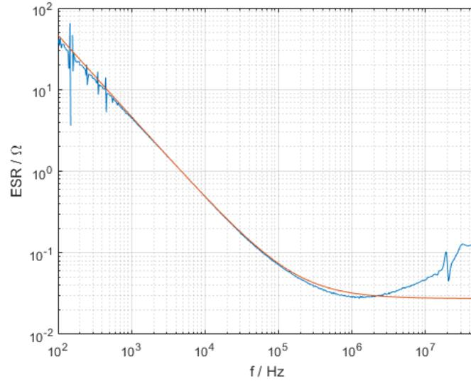
Figure 4.7: Measured and modelled ESR of an FDCC. Blue: measured ESR; red: modelled ESR
