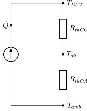
Figure 6.4: Equivalent thermal circuit of the CMS
