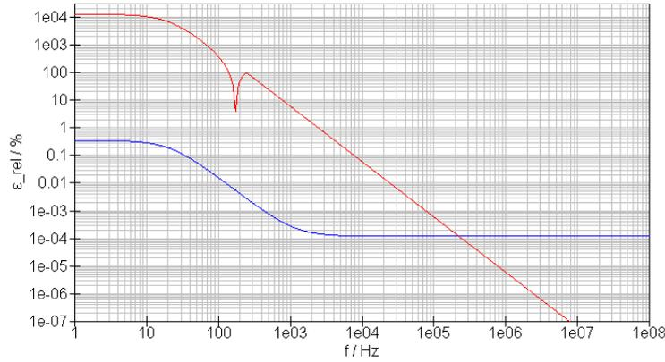
Figure 4.6: Simulation of the relative ESR error (red) and the relative capacitance error (blue)
