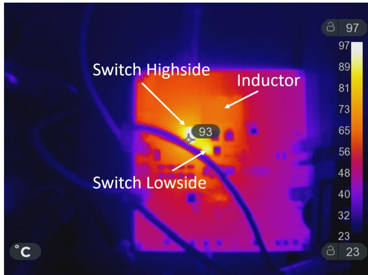
Figure 6.10: Thermal image of the buck converter on the evaluation board during the 495 kHz measurement
