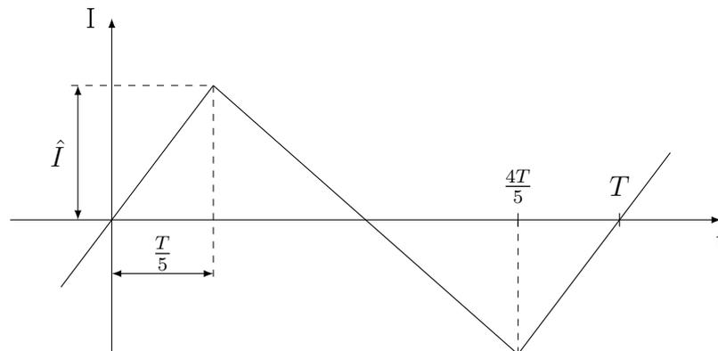
Figure 6.12: Inductor current of an ideal buck converter
