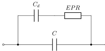
Figure 1.5: Parallel equivalent circuit model of an FDCC
