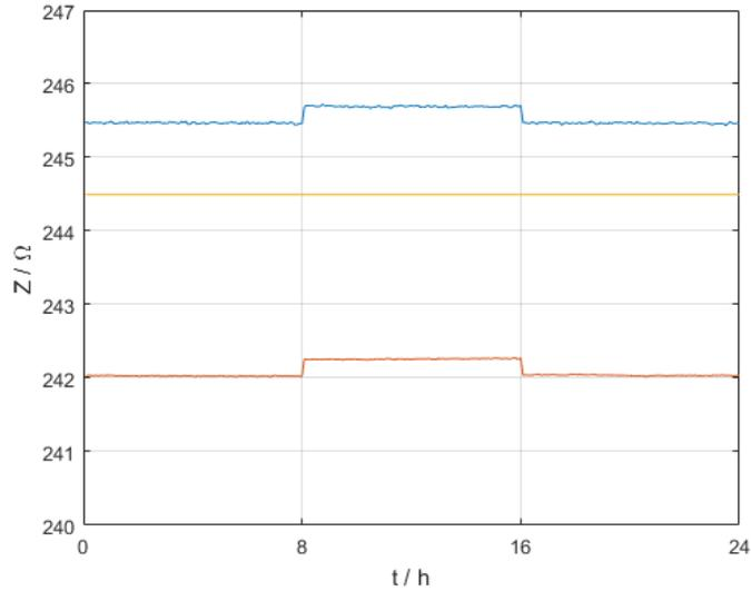
Figure 4.11: Magnitude of the C0G capacitor over time. Blue: measurement bridge; red: TCM divided by two; yellow: ideal
