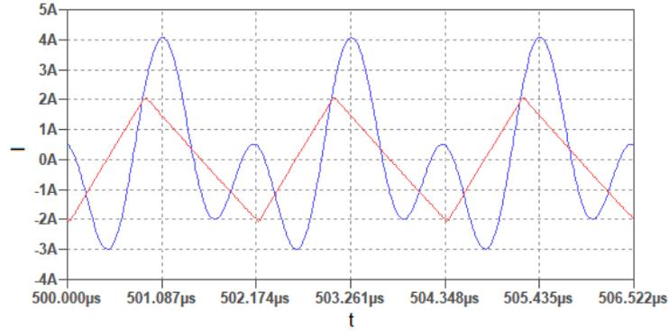
Figure 6.16: Simulated current of the output capacitor (blue) and output capacitor current of an ideal buck converter (red)
