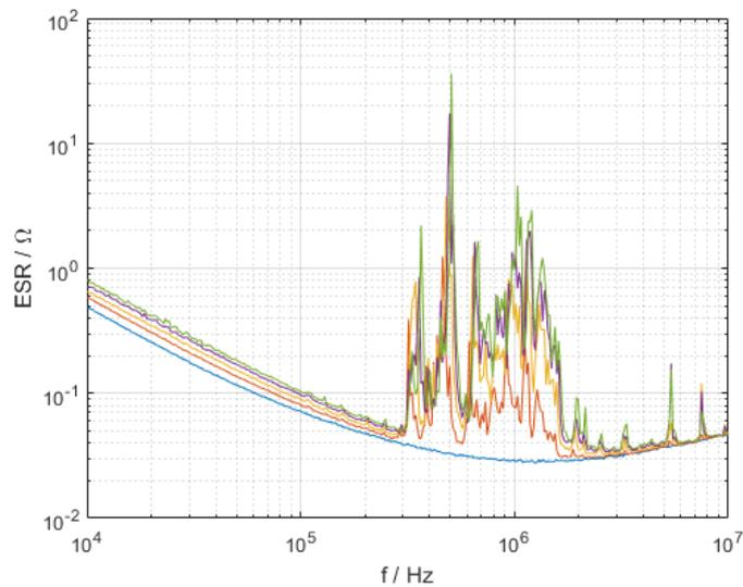
Figure 5.5: ESR versus frequency with dc bias. Blue: 0 V dc bias; red: 150 V; yellow: 300 V; violet: 450 V; green 600 V
