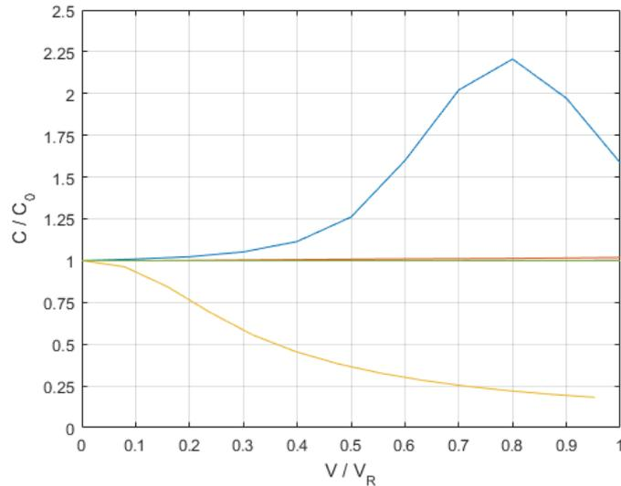
Figure 5.3: Relative capacitance change of capacitors with dc bias. The capacitance is referred to the capacitance without dc bias. The voltage is referred to the rated voltage. Blue: CeraLink; red: e-cap; yellow: X7R; violet: film; green: C0G
