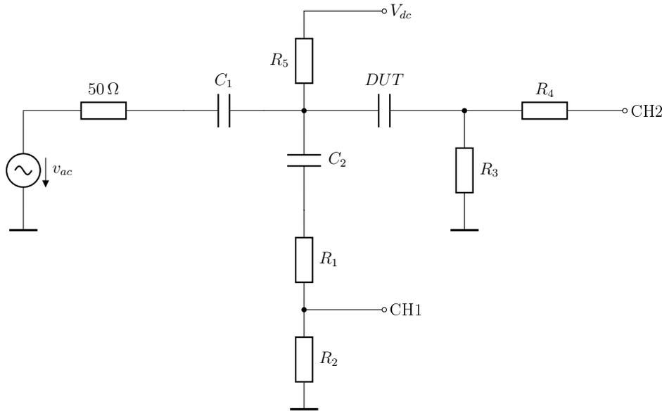
Figure 8.1: Circuit of the impedance measurement bridge
