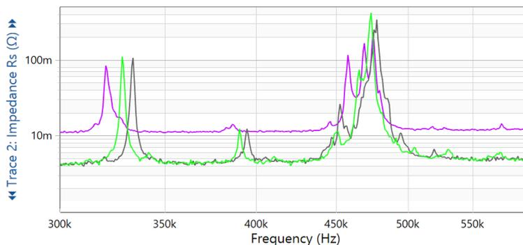
Figure 6.6: Resonances of three FDCCs of the same type with matching PR
