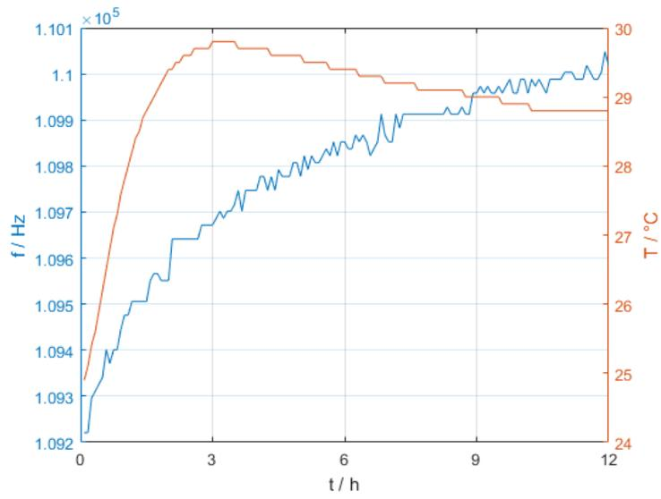
Figure 5.7: PR frequency (blue) and ambient temperature (red) over time after attaching dc bias
