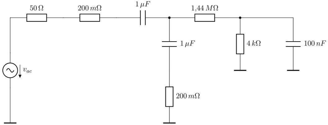
Figure 3.4: Schematic of the error simulation of the TCM
