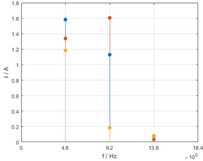
Figure 6.18: Fourier coefficients measured (blue), simulated (red) and calculated (yellow)
