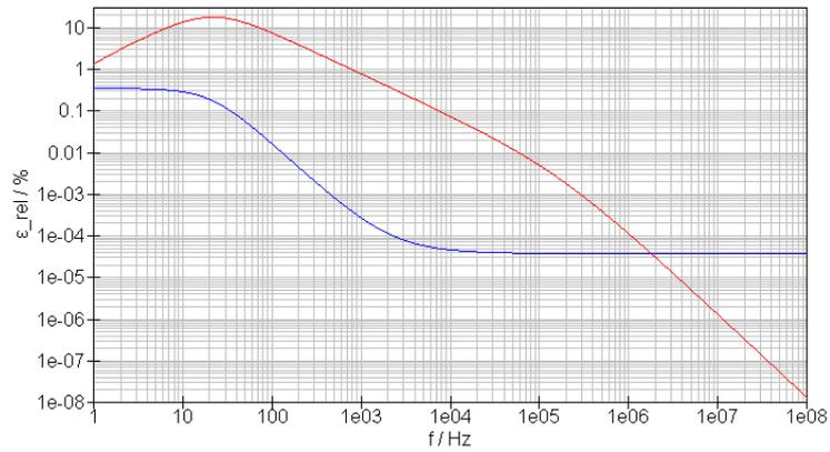
Figure 4.8: Simulation of the relative ESR error (red) and the relative capacitance error (blue) of an FDCC
