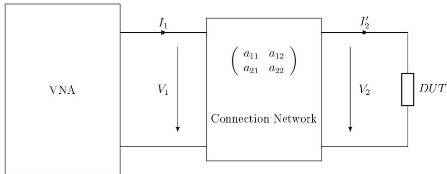
Figure 2.1: Impedance measurement circuit with an arbitrary connection network
