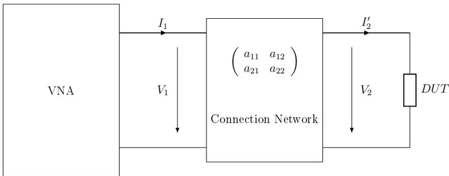
Figure 8.5: Impedance measurement circuit with an arbitrary connection network
