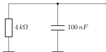
Figure 3.3: Output impedance model of the used voltage source
