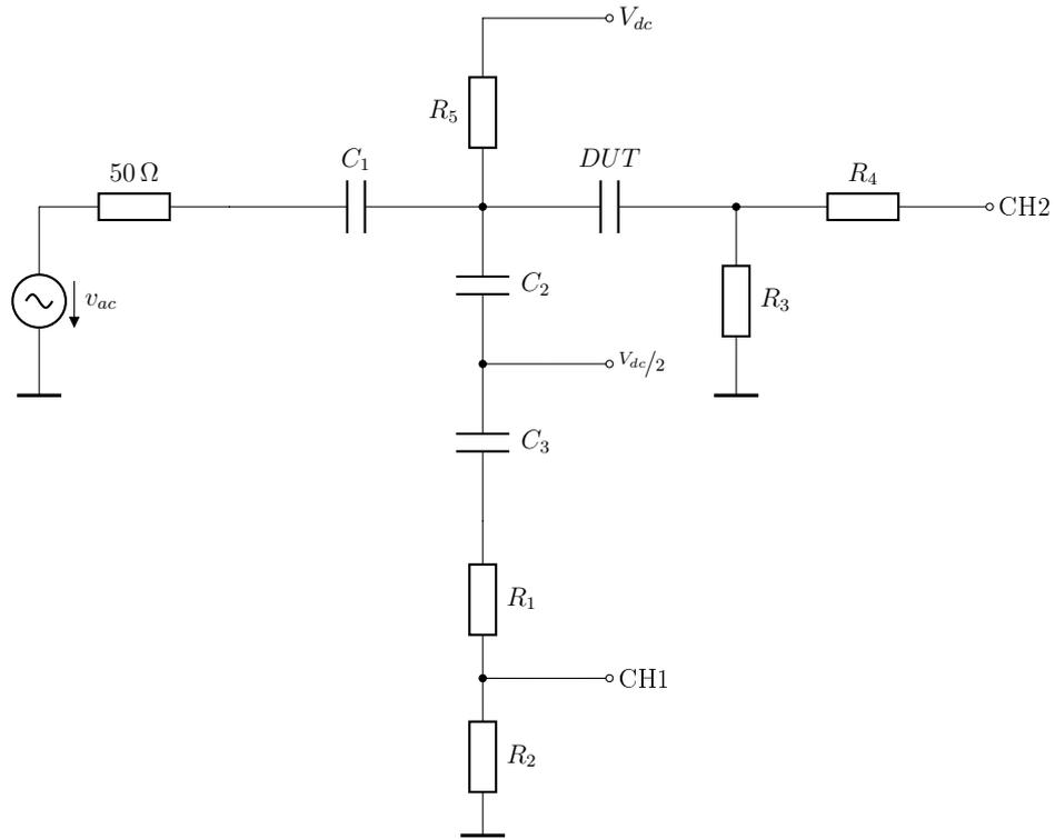
Figure 4.10: Possible circuit for a dc biased OSL calibration
