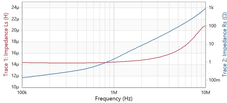
Figure 6.13: Measured inductance (red) and ESR (blue) of the inductor in the buck converter
