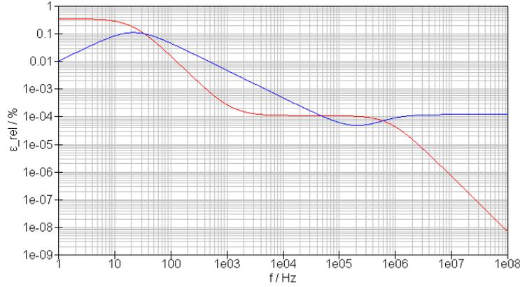
Figure 4.5: Simulation of the relative magnitude error (red) and the relative phase error (blue)
