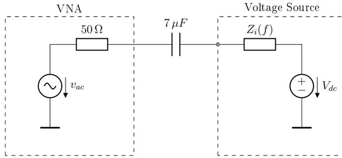
Figure 3.1: Measurement setup for the output impedance measurement of a voltage source
