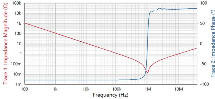
Figure 1.3: Bode plot of a capacitor. Red: magnitude; blue: phase
