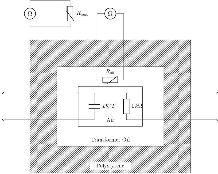
Figure 6.3: Schematic of the improved CMS
