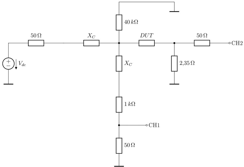
Figure 4.1: Schematic of the parameter sweep simulation
