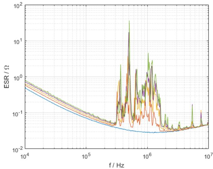
Figure 8.3: ESR versus frequency with dc bias. Blue: 0 V dc bias; red: 150 V; yellow: 300 V; violet: 450 V; green 600 V
