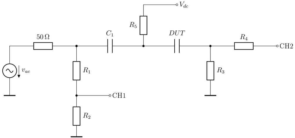
Figure 3.7: Circuit of a possible impedance measurement bridge
