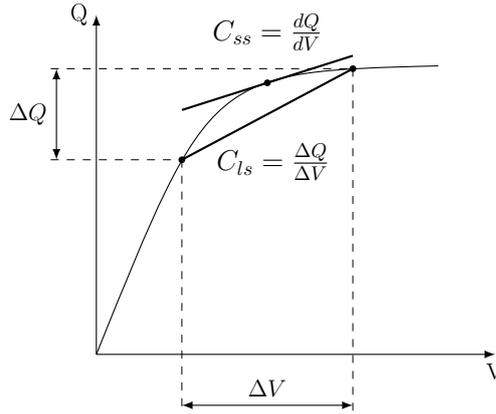
Figure 1.4: Difference between small signal and large signal capacitance
