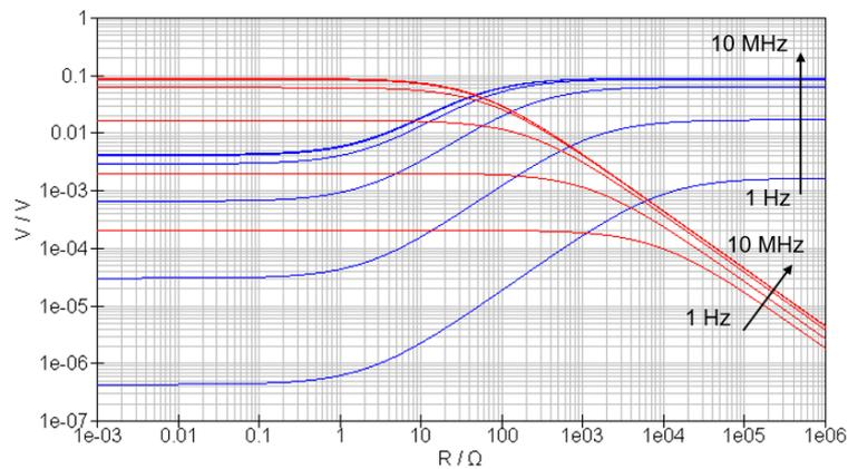
Figure 4.2: Simulation of the voltage against the impedance of CH1 (blue) and CH2 (red)
