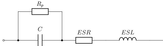
Figure 1.1: Equivalent circuit of a real capacitor
