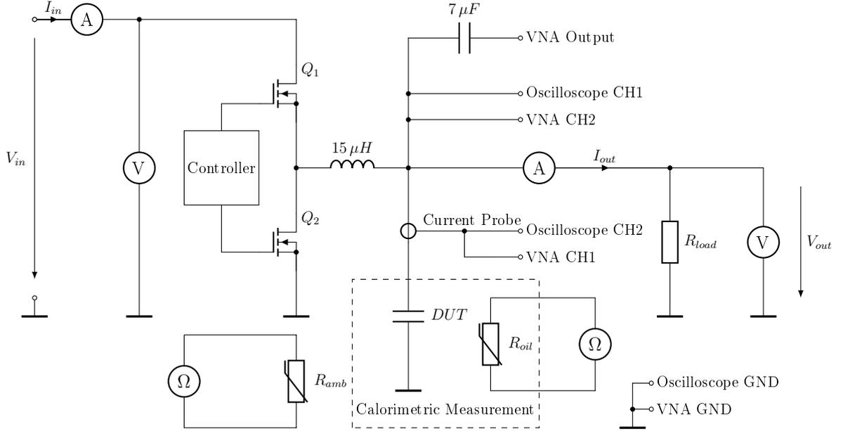
Figure 6.5: Capacitor loss measurement setup: measurement of the input and the output power with two ampere meters and two voltmeters, the ESR with the PR with the VNA, the voltage and current of the output capacitor with the oscilloscope and the capacitor losses with the two ohmmeters and the two temperature dependent resistors
