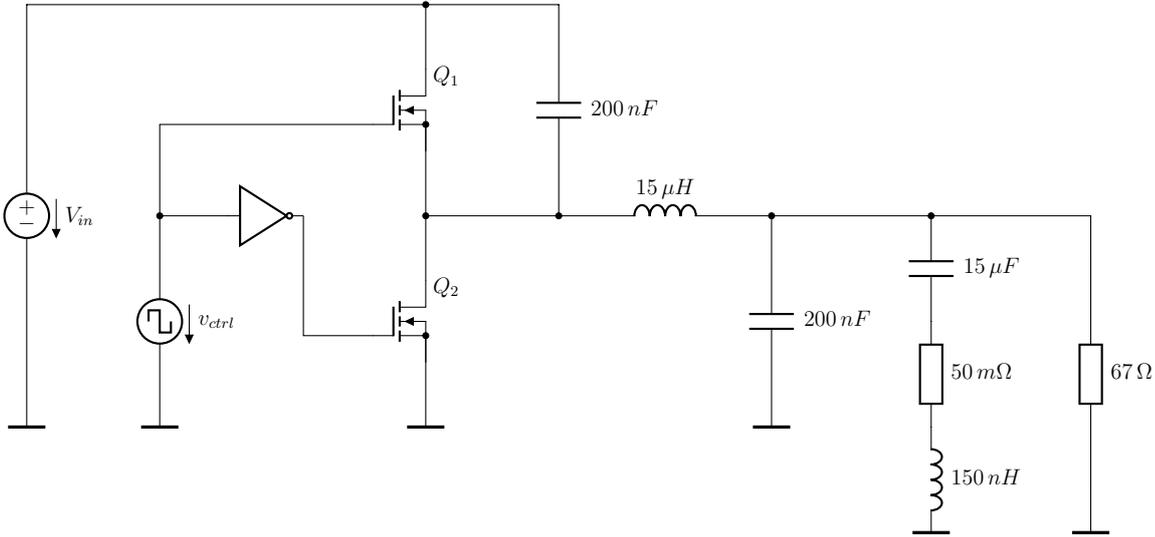
Figure 6.15: Schematic of the capacitor current simulation
