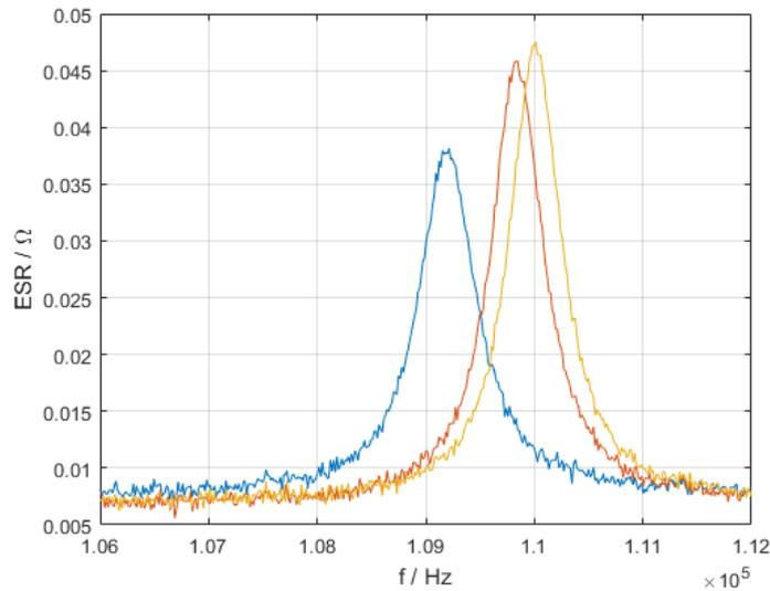
Figure 5.6: PR frequency after attaching dc bias. Blue: initial; red: after 6 hours; yellow: after 12 hours
