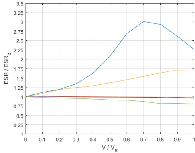
Figure 8.2: Relative ESR change of capacitors with dc bias. Blue: CeraLink; red: electrolytic capacitor; yellow: X7R; violet: film; green: C0G
