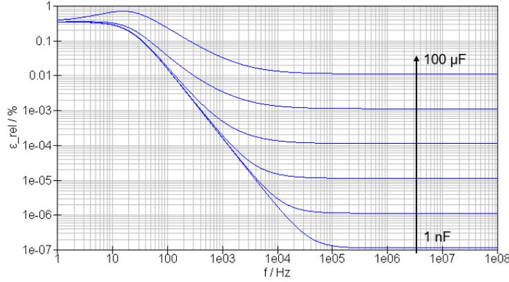
Figure 4.9: Simulation of the relative capacitance error over frequency and capacitance
