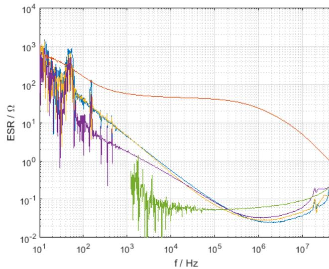
Figure 5.2: ESR of capacitors versus frequency without dc bias. Blue: CeraLink; red: e-cap; yellow: X7R; violet: film; green: C0G
