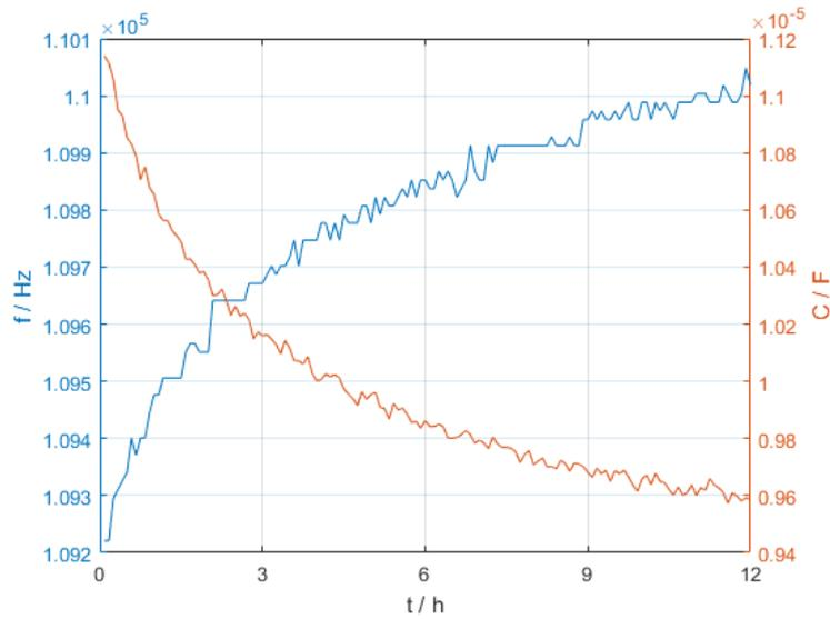
Figure 5.8: PR frequency (blue) and capacitance (red) over time after attaching dc bias
