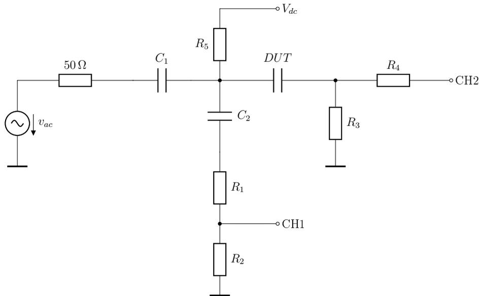
Figure 3.8: Circuit of the improved impedance measurement bridge
