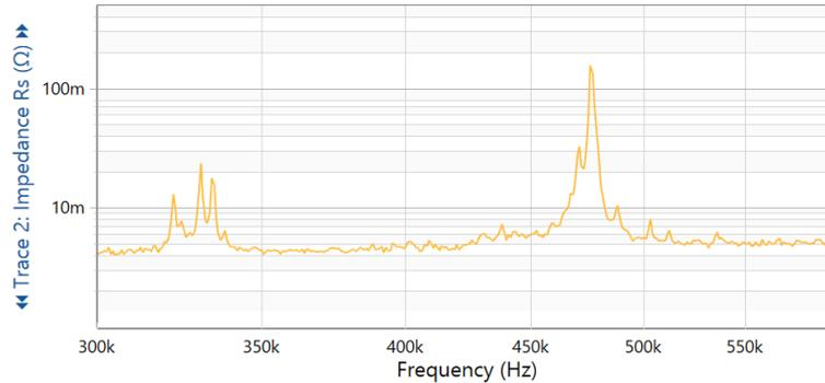
Figure 6.7: Resonances of the parallel circuit of three FDCCs with matching PR
