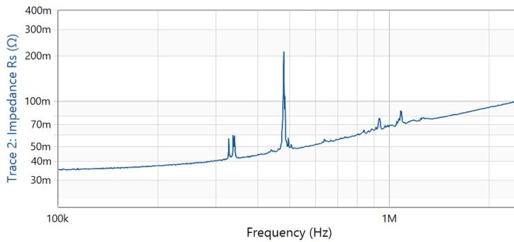
Figure 6.19: ESR of the capacitor inserted in the cage
