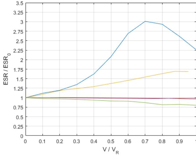
Figure 5.4: Relative ESR change of capacitors with dc bias. The ESR is referred to the ESR without dc bias. The voltage is referred to the rated voltage. Blue: CeraLink; red: e-cap; yellow: X7R; violet: film; green: C0G
