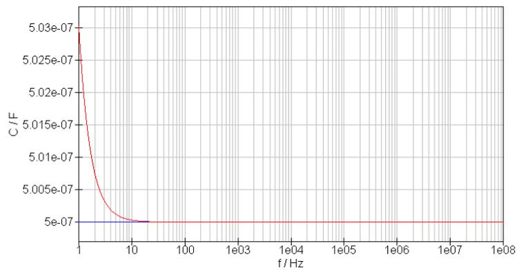
Figure 3.5: Simulated capacitance of the TCM. Red: simulation of the measured capacitance; blue: ideal capacitance
