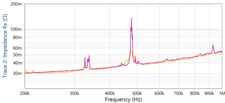
Figure 6.2: PR of a capacitor in air (pink) and in oil in the CMS (orange)
