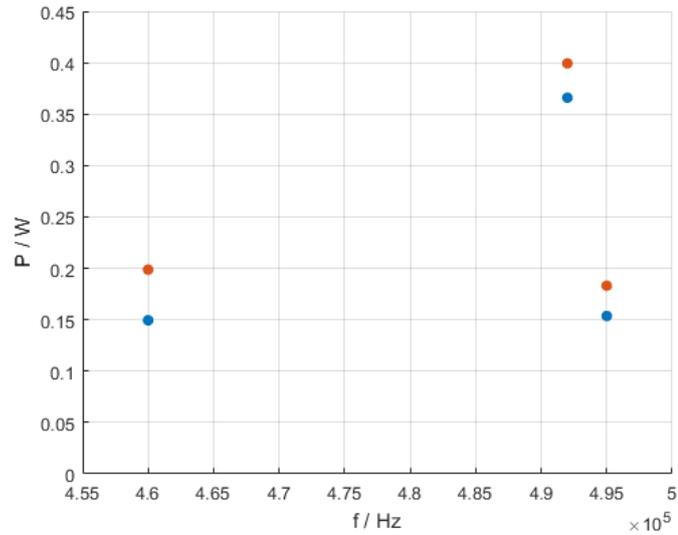
Figure 8.4: Measured and calculated losses of the output capacitor for the three measurement points. Blue: measured losses; red: calculated losses
