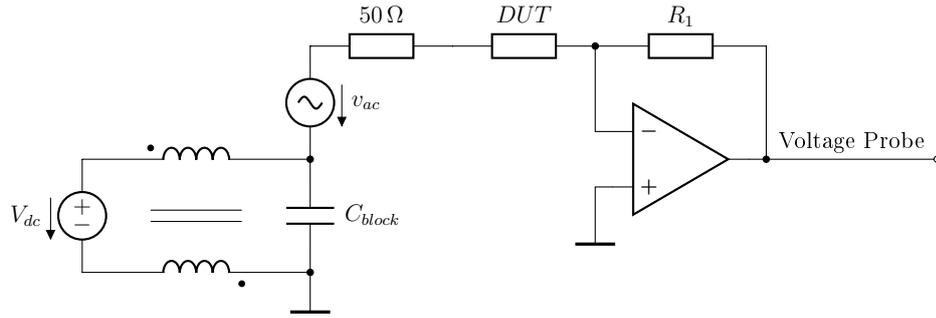
Figure 2.2: Series circuit of an ac and a dc voltage source and current measurement with an ABB
