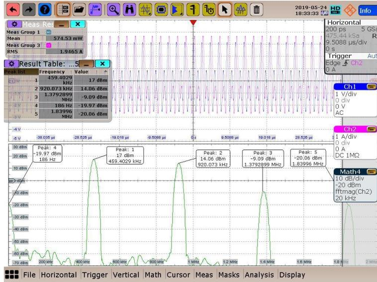
Figure 6.17: Oscilloscope measurement at 460 kHz. Top: voltage, current and instantaneous power of the output capacitor in time domain; bottom: spectrum of the capacitor current
