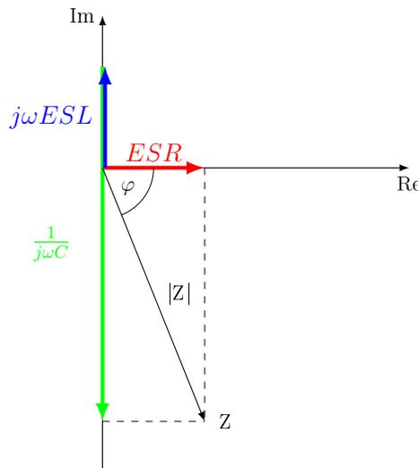
Figure 1.2: Impedance of a real capacitor in the complex plane
