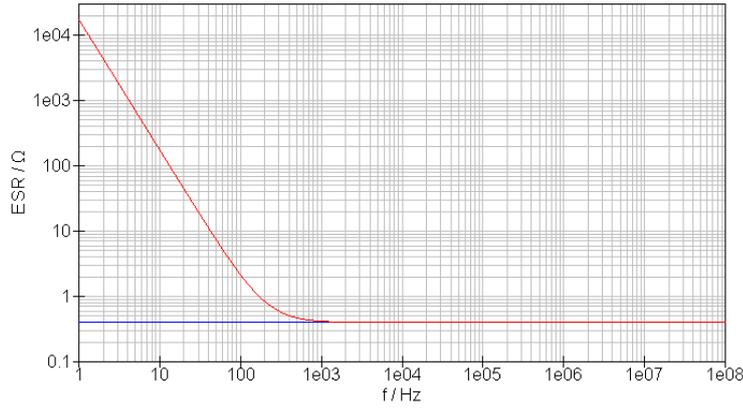
Figure 3.6: Simulated ESR of the TCM. Red: simulation of the measured ESR; blue: ideal ESR
