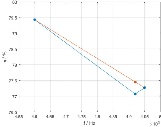
Figure 6.9: Efficiency of the converter at the three measurement points (blue) and interpolation with expected efficiency without PR (red)
