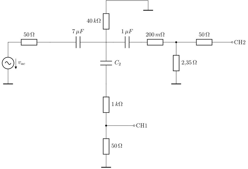
Figure 4.4: Schematic of the error simulations
