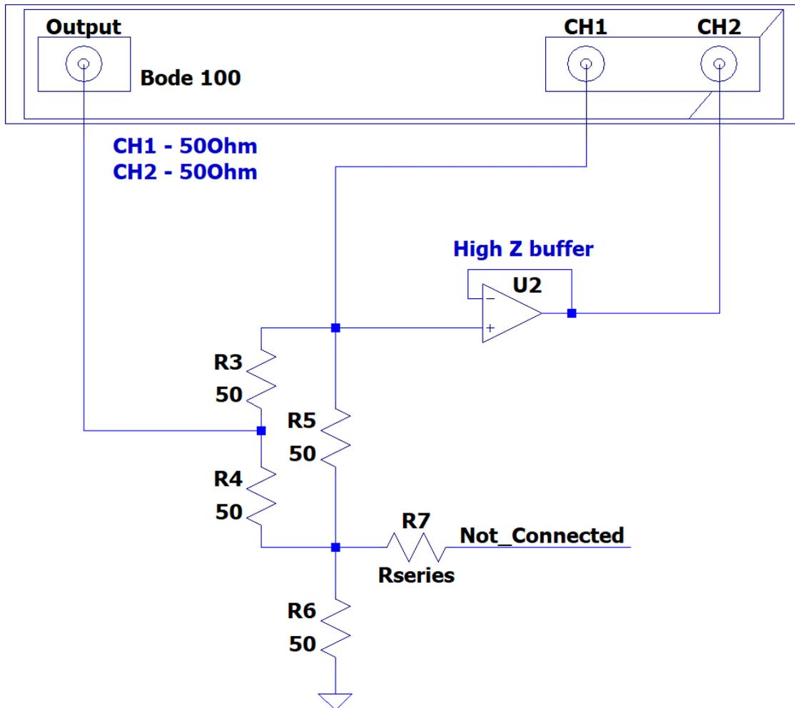
Figure 22 Calibration connection
