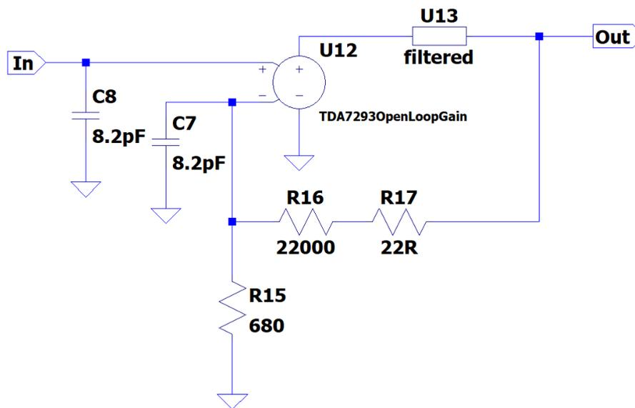
Figure 28 The amplifier model, with inclusion of feedback resistors
