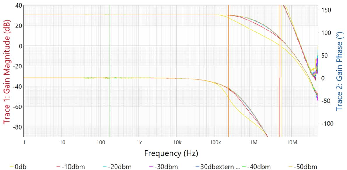
Figure 3 Effect of input signal amplitude on signal gain measurement
