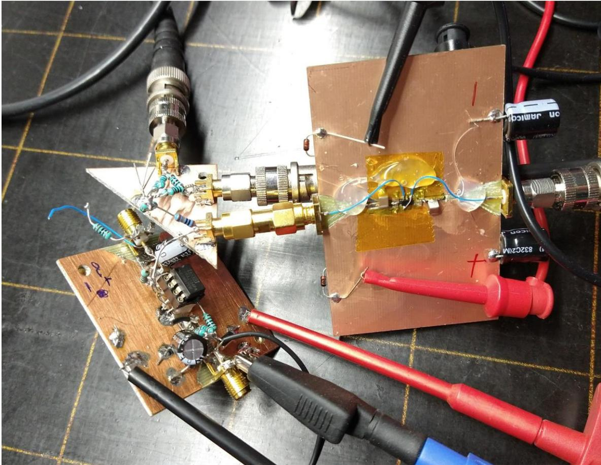
Figure 25 Input capacitance measurement setup
