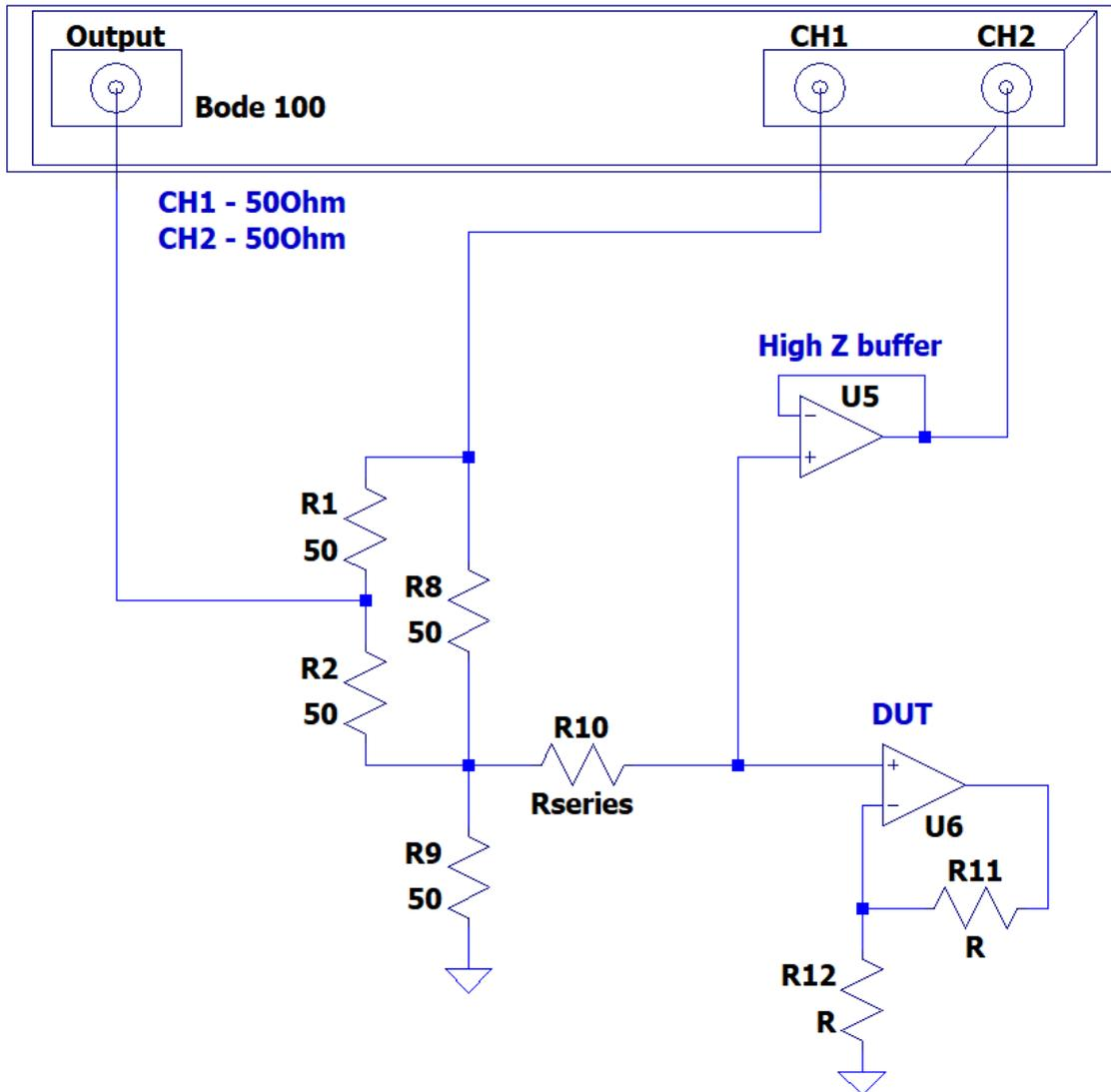
Figure 23 DUT connection
