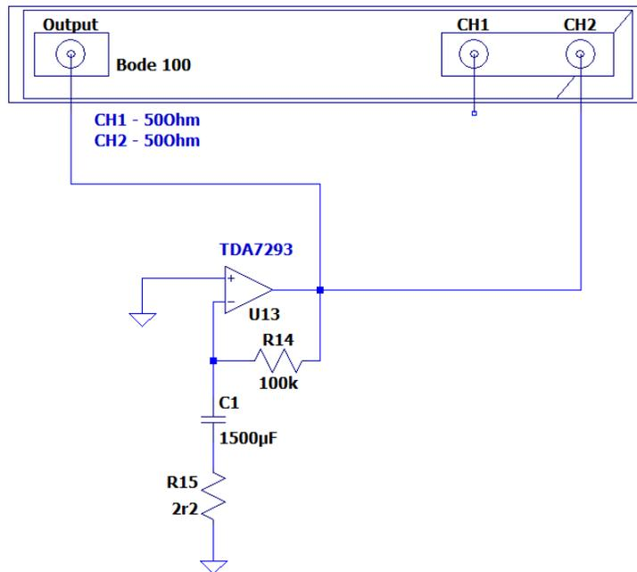
Figure 17 Output impedance measurement with filtered feedback
