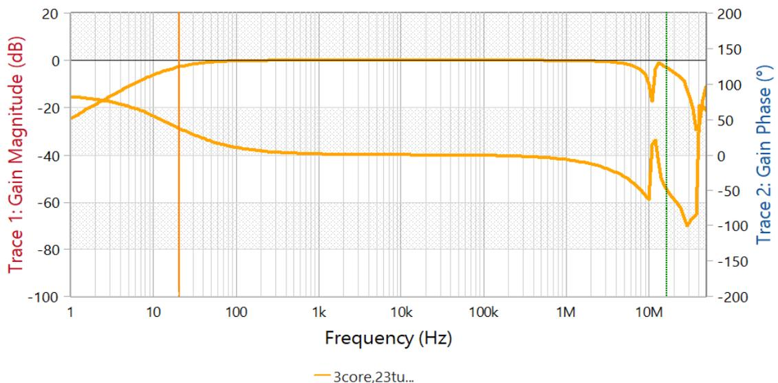
Figure 8 DIY Injection transformer transfer function
