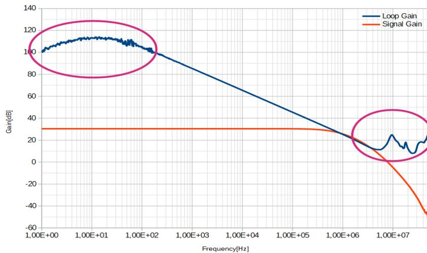
Figure 7 Loop gain and signal gain measurement
