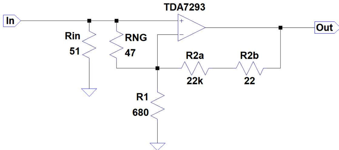
Figure 9 Modified amplifier circuit
