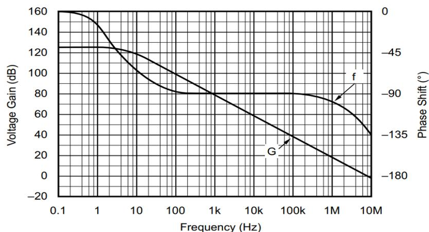
Figure 1 Open loop gain of OPA2134, courtesy of the part datasheet
