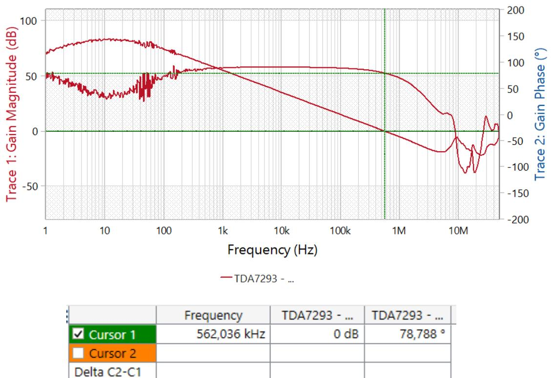
Figure 6 Loop gain measurement
