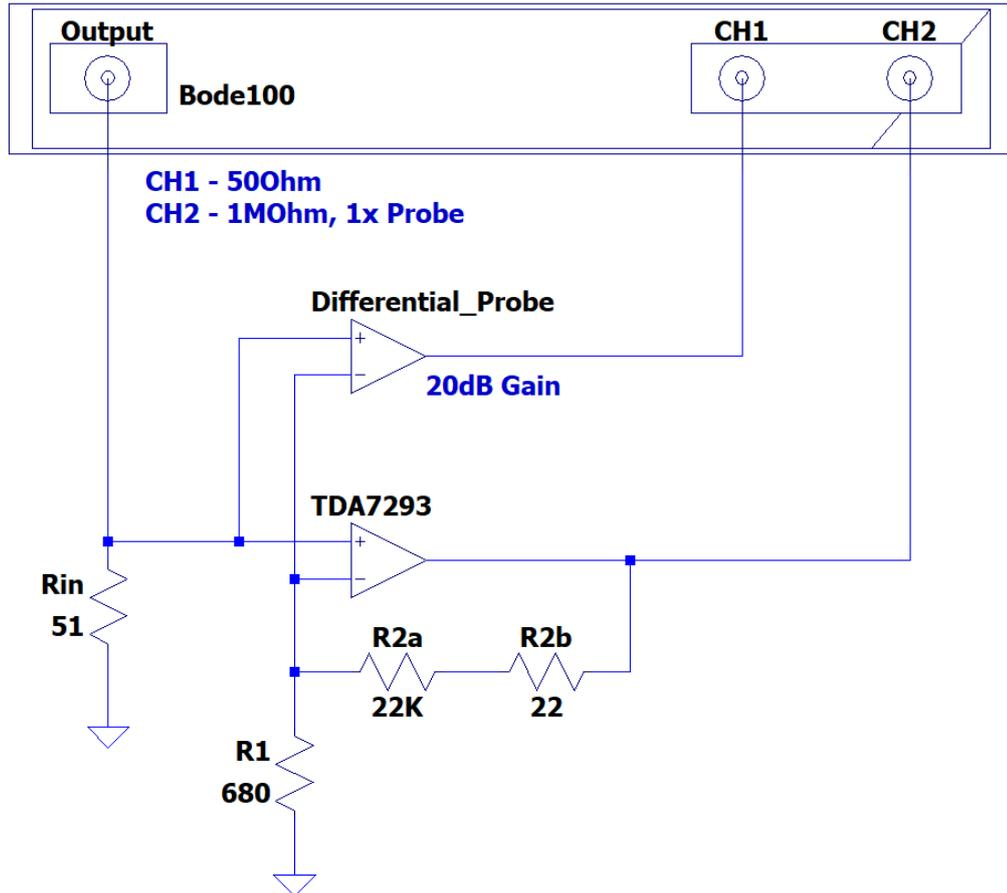
Figure 13 Differential connection of our amplifier
