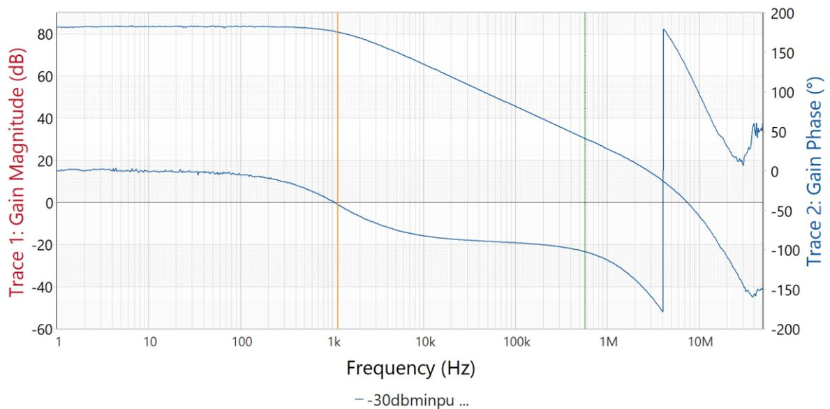
Figure 14 Open loop gain measurements with differential probe
