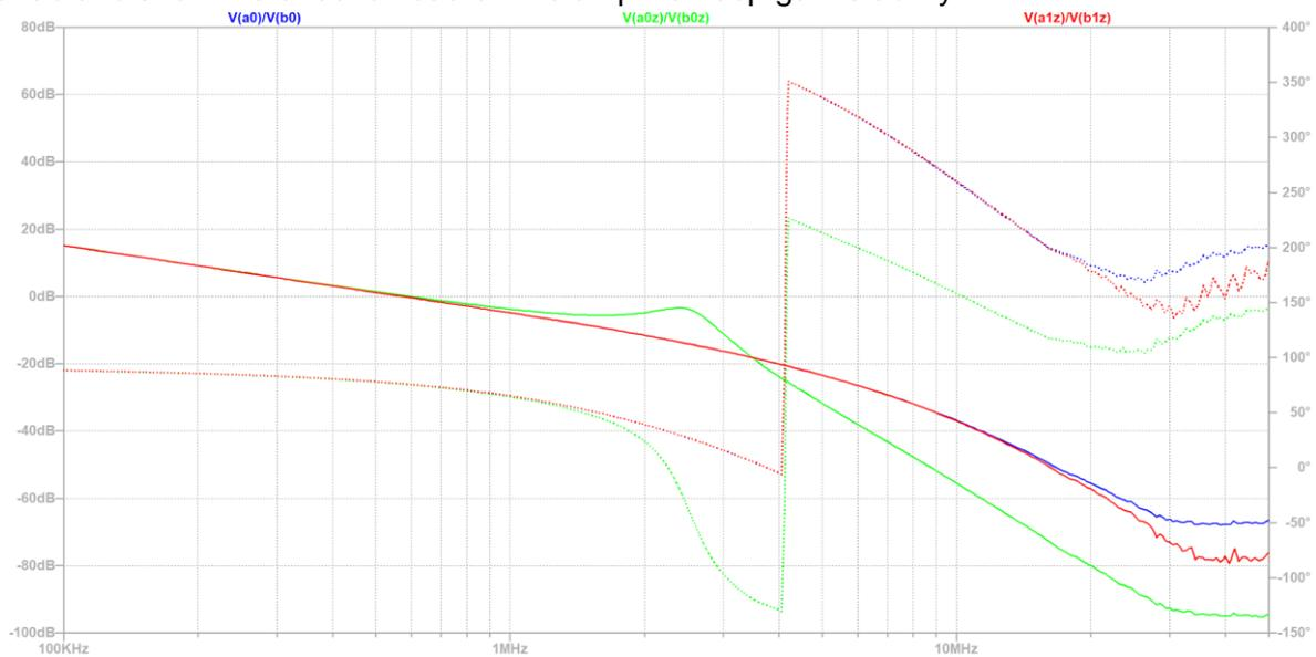
Figure 30 Effects of load capacitance on loop gain
