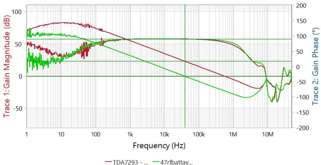
Figure 10 Loop gain of modified circuit
