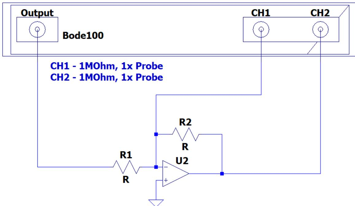
Figure 12 Loop Gain measurement of inverting amplifier
