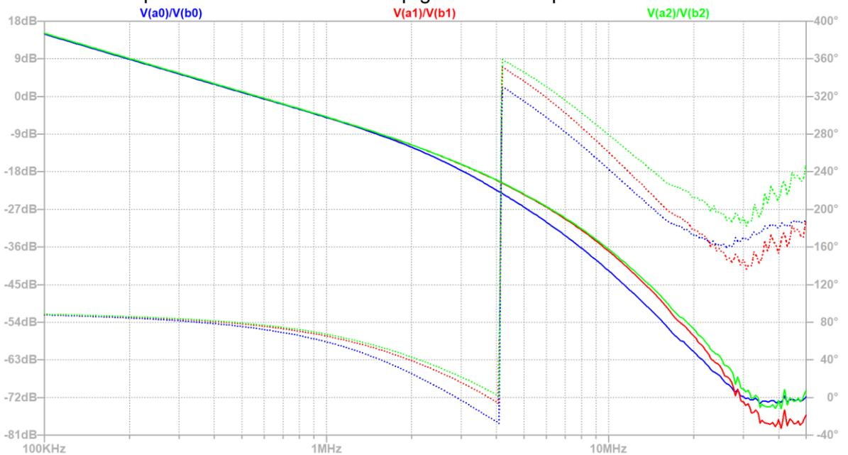
Figure 29 Effect of model on loop gain with 8 Ohm load
