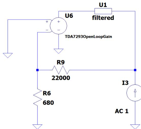
Figure 19 Closed loop output impedance simulation
