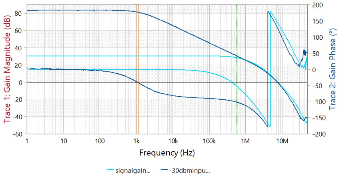
Figure 15 Open loop gain and signal gain
