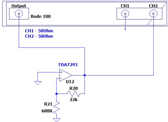
Figure 16 Closed Loop output impedance measurements
