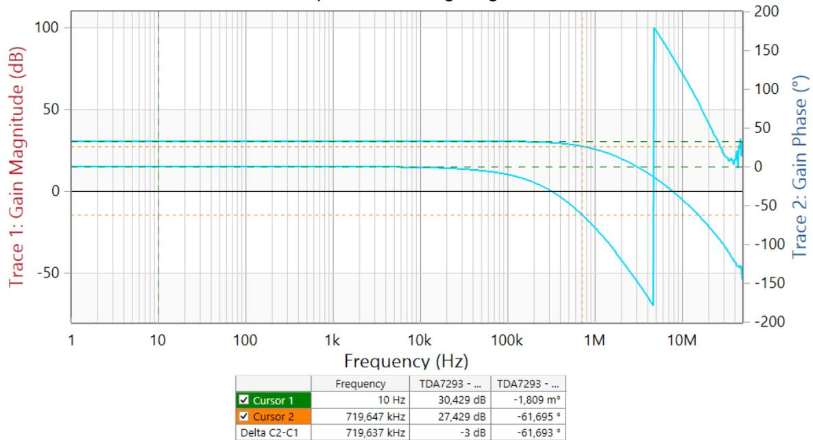
Figure 5 Amplifier signal gain/closed loop gain
