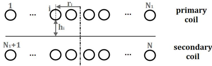
Figure 3: Configuration of the primary and secondary coil
