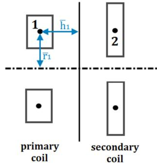
Figure 4: Cross section of the coils. Filaments for the first order approximation
