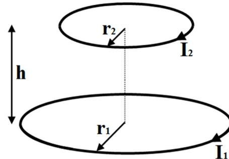
Figure 1: Two coaxial circular filaments in free space
