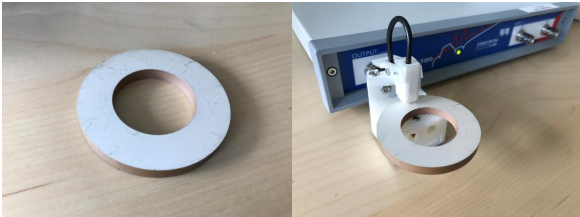
Fig. 23 Ring sample (left), sample in the TOOsonix fixture (right)
