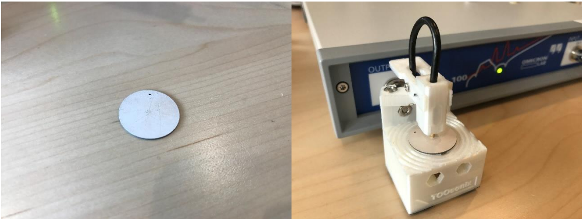
Fig. 18 Disc sample - material B (left), sample in the TOOsonix fixture (right)
