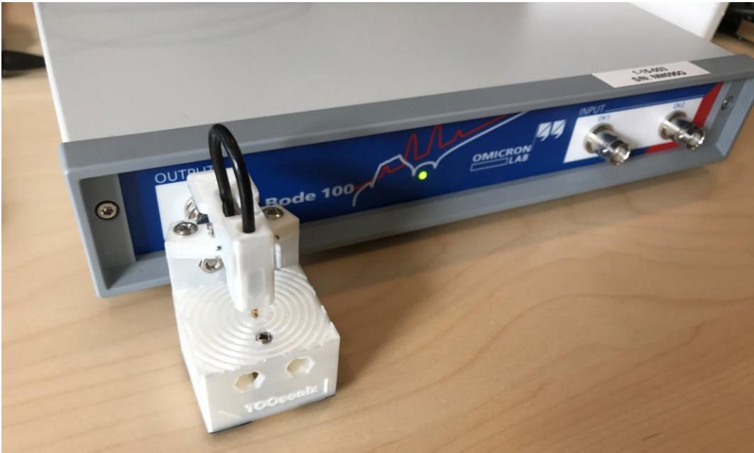
Fig. 6 Bode100 with the test fixture
