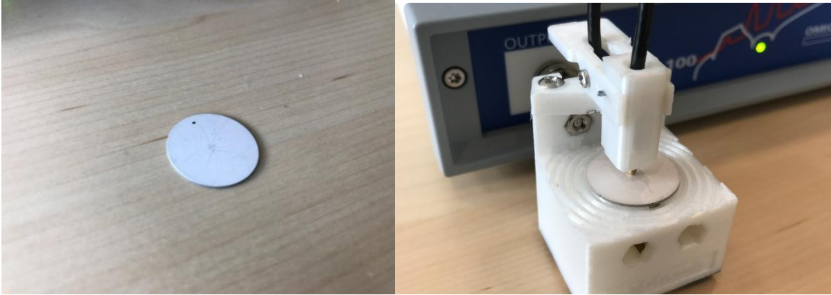
Fig. 13 Disc sample - material A (left), sample in the TOOsonix fixture (right)
